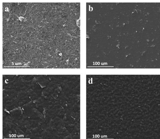
Figure (present in the paper). SEM images of the surfaces of PDMS films coated with (a) CNTs, (b) GE, (c) GO, and (d) rGO by spray coating. The carbon nanomaterial concentration for all of the spraying dispersions was 0.075 mg/mL.
