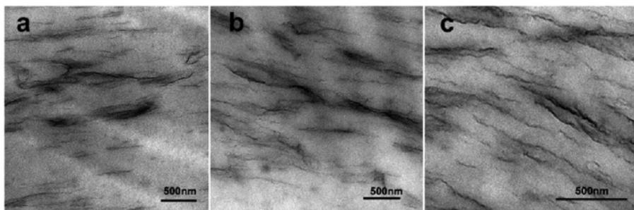
*Figure (present in the paper). Transmission electron microscope cross-sectional images of chitosan composite films for (a) CS/GO-T, (b) CS/B/IGO and (c) CS/B/IGO-T.*
