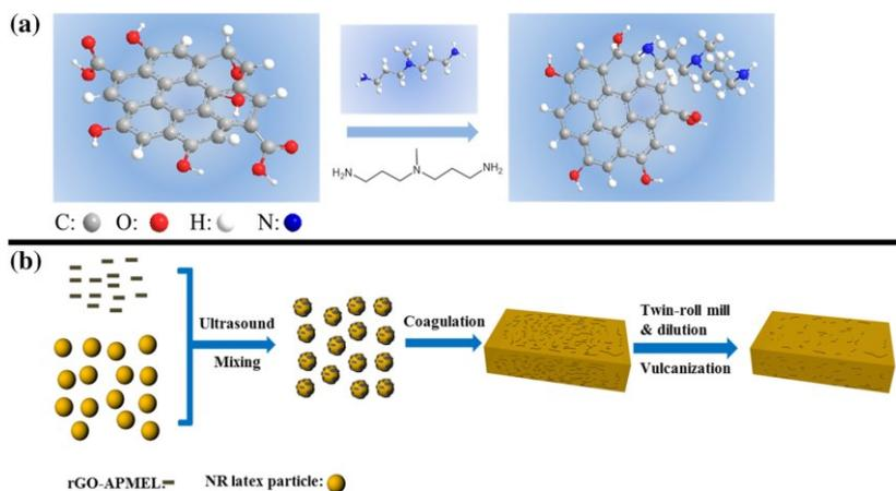
Scheme 1 (present in the paper). Scheme 1. (a) Functionalization of GO by grafting reaction with APMEL and (b) preparation of NR/rGO composites through a latex mixing using the APMEL-functionalized GO aqueous dispersion.
