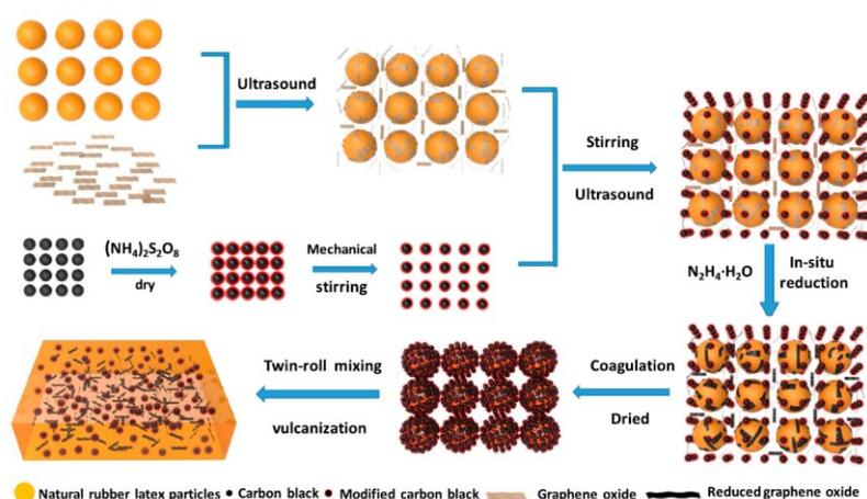
Scheme 1 (present in the paper). WCL method for the preparation of rGO/CB/NR composites.
