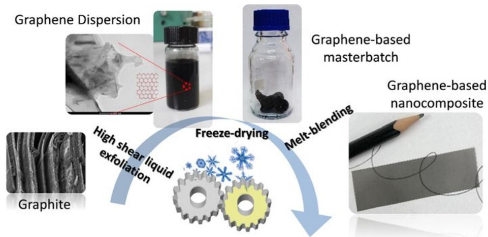
Graphical Abstract: Schematization of process from graphite to graphene dispersion, graphene masterbatch up to graphene-based nanocomposite.
