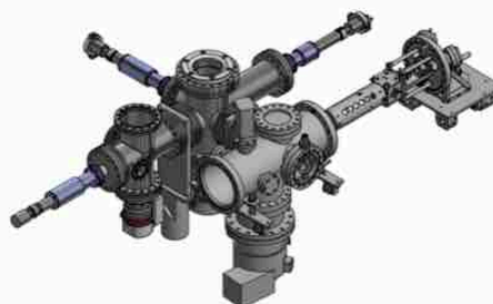
Figure 2. The deposition chamber (Ionvac Process srl) connected to the ESI source.
