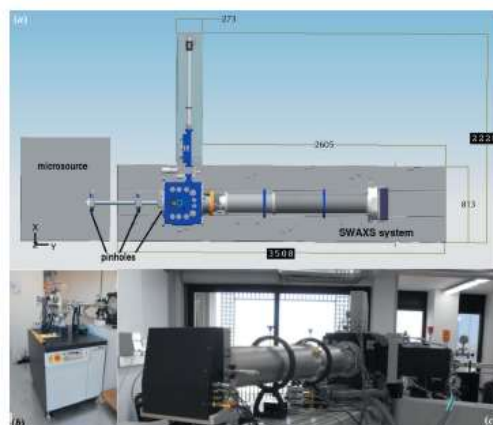
Figure 1 (a) Scheme of the XMI-LAB; (b) Fe-Eu SuperBright microsource; (c) SAXS/WAXS (SWAXS) three-pinhole camera.
