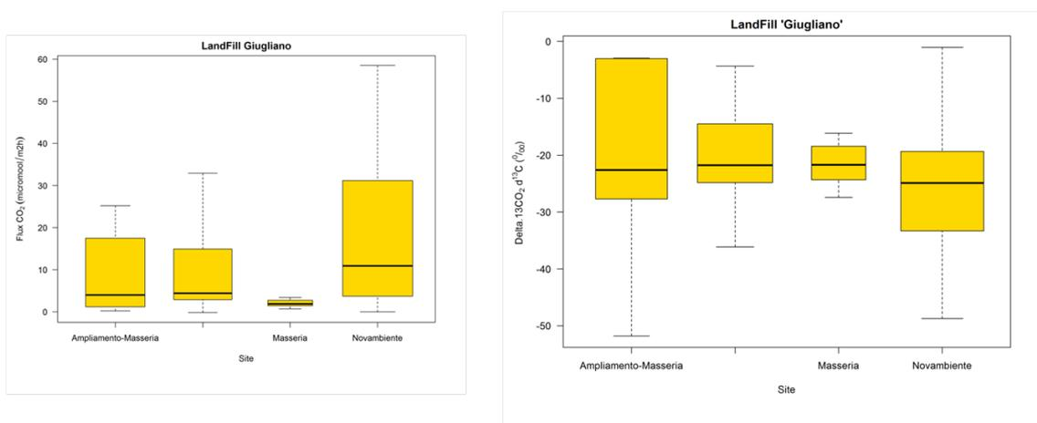
Figure 6 Box plots of CO<sub>2</sub> and  $\delta^{13}\text{C}$  fluxes measured at the Giugliano's Landfill during 2015-2016.
