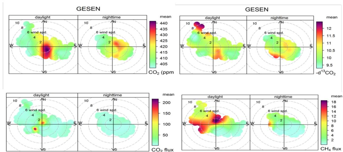
Figure 4 Polar plots of atmospheric concentrations and turbulent fluxes measured at the Gesen Tower (20 m. a.g.l.) between July and September 2016.
