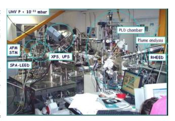
complementary surface sensitive techniques. A UHV distribution chamber is employed to transfer the samples between the load-lock fast entry, the pulsed laser deposition chamber and the analysis chambers.
