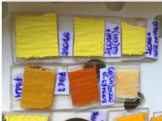
Series of artificially aged oil paint mock-ups prepared using different types of cadmium sulfide-based pigments. Photo Credit: Letizia Monico (CNR-SCITEC, Italy).
