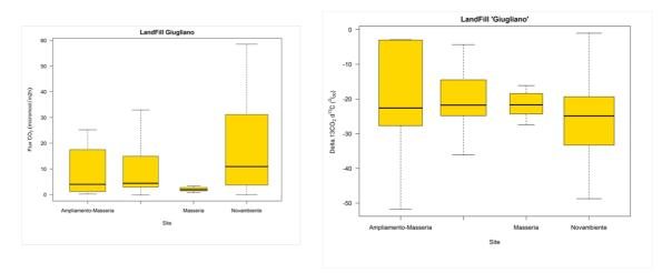
Figure 6 Box plots of CO<sub>2</sub> and  $\delta^{13}$ C fluxes measured at the Giugliano's Landfill during 2015-2016.
