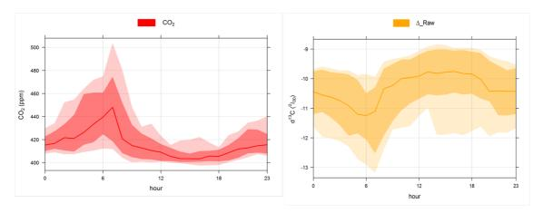
Figure 5 Daily cycles of  $CO_2$  concentrations and  $\delta^{13}C$  ratio continuously measured at Gesen tower between July and September 2016.
