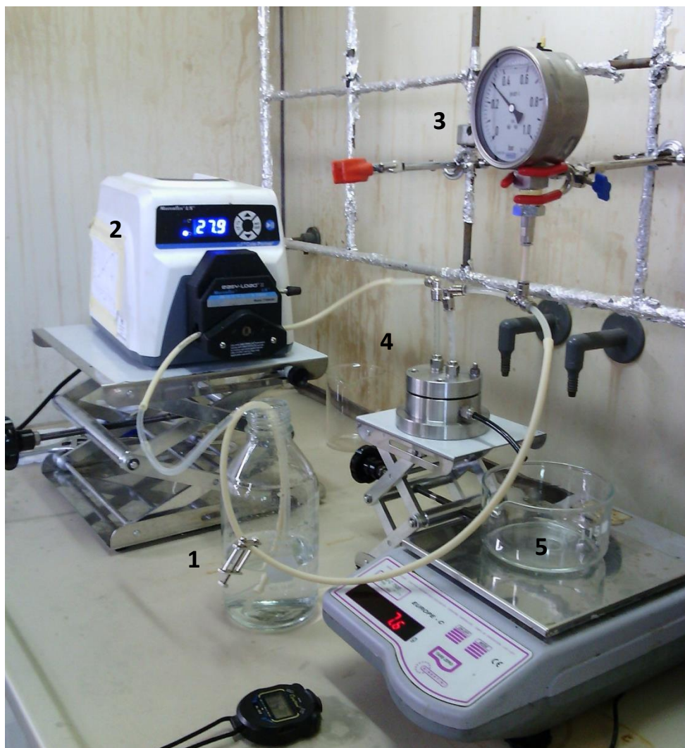
Figure 3. Assembly of the ultrafiltration system: 1) feed/retentate, 2) peristaltic pump, 3) manometer, 4) cross-flow membrane cell, 5) permeate
