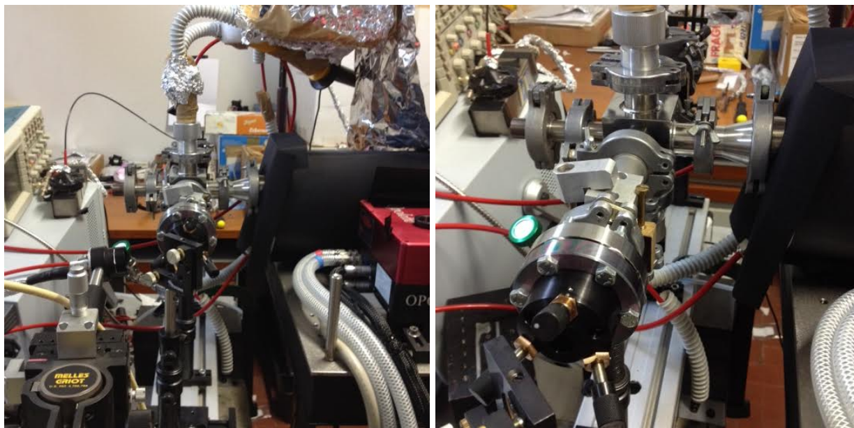
Experimental Apparatus. Discharge chamber with CRDS mirror mounts.
