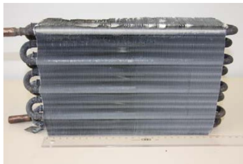
Figure 1: Fin-tube heat exchanger coated by PST method with SAPO34.
