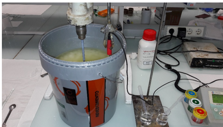
Figure 9. Residual DAC oxidation by \text{NaClO}_2 .
