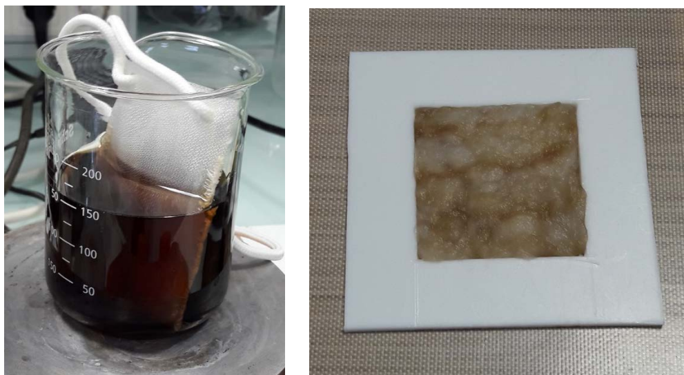
Figure 20. Submersion of DCC in SL (right); Aspect of DCC (PSL) 1 after LbL deposition.
