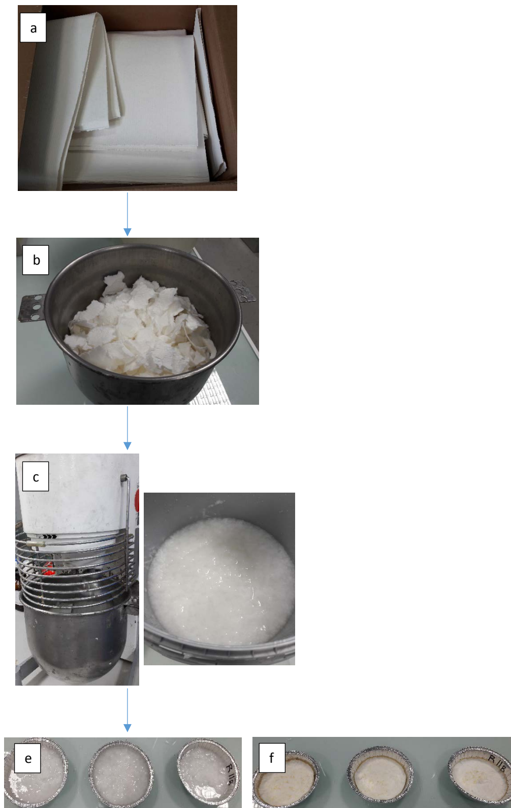
Figure 1. Phases of cellulose disintegration and oxidation: from pine cellulose sheet to DAC.
