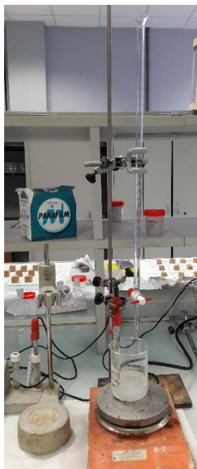
Figure 4. Titration of aldehyde content in DAC.
