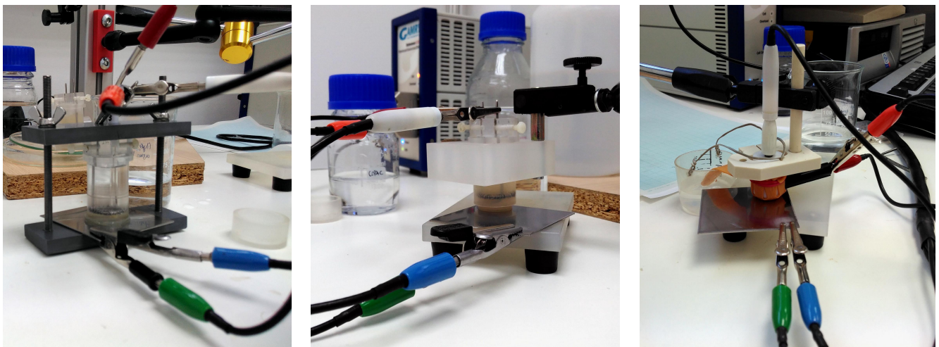
Figure 1 - Measurement setup (from left to right): Standard Cell (STD); Gel Cell (GP); Contact Probe (CP).
