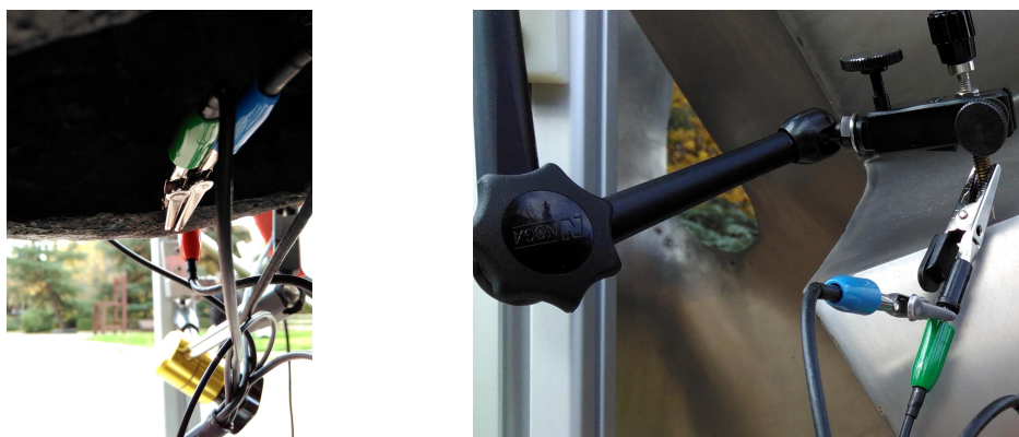
Figure 4 - WE contact methods: alligator clip on scratched hidden area on bronze (left); pressure pin on stainless steel (right)
