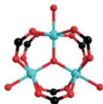
Figure 3. Structure of the Iron-based inorganic SBU [Fe 3 (μ 3 -O)(RCOO) 6 ].
