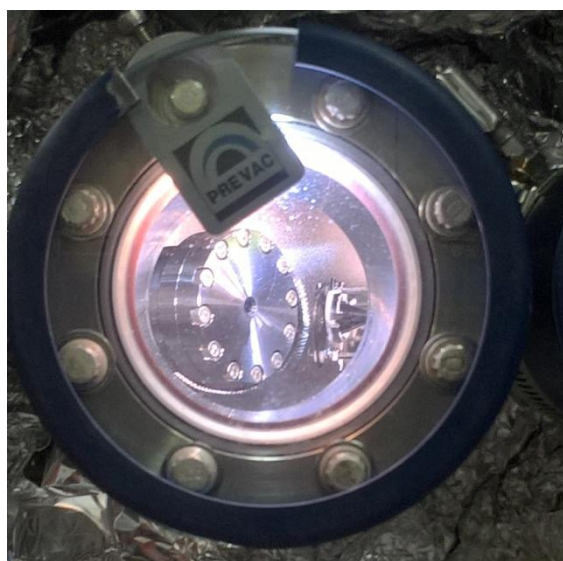
Figure 8. Micro-fluidic cell in the UHV experimental chamber
