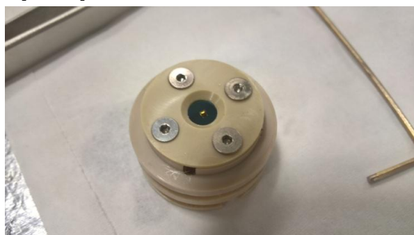
Figure 2. Image of the static liquid cell.
