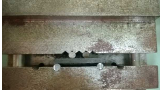
Figure 13 – Composite sample under four point bending
