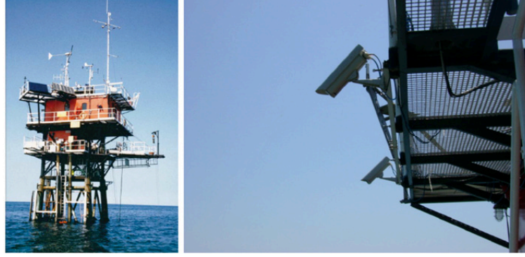
Fig. 2: The “Acqua Alta” oceanographic tower (left), and the WASS stereo-photogrammetric system (right).
