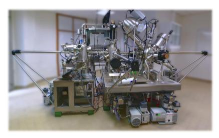
The experimental setup has been conceived to allow the study solid/gas interfaces well as solid/liquid interfaces. As seen in the figure below, the apparatus consists of a Scanning Tunnelling Microscopy (STM), an Atomic Force Microscopy (AFM) complemented by Hemispherical Analyser for x-ray electron spectroscopy (XPS). preparation chamber hosts an ion gun,
