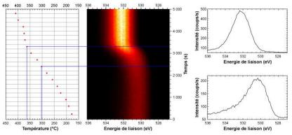
core level measurement taken on CuAl(111) during the oxidation at about  $10^{-5}$  mbar of molecular oxygen as a function of the sample temperature. As can be seen from the figure in the middle a clear phase transition occurs in the temperature range from 300°C to 360°C: while a simple adsorption of the
