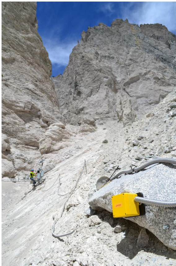
Figure 2 – The geophone A (left) at the downstream station and the geophone B (right) installed at the bridge section.
