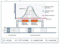
The bypass is designed in a way that flow thru the sensor and the bypass is always proportional to the flow range for which the mass-flow controller is built.
