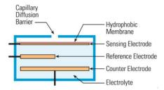
Gas that comes in contact with the sensor first passes through a small capillary-type opening and then diffuses through a hydrophobic barrier, and eventually reaches the electrode surface. This approach is adopted to allow the proper amount of gas to react at the sensing electrode to produce a sufficient electrical signal while preventing the electrolyte from leaking out of the sensor.
