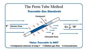
The emission rate of a permeation tube is dependent on the following factors: physical characteristics of its permeable membrane, permeability of its chemical analyte through the membrane, temperature of the permeation tube and partial pressure across its permeable membrane.
