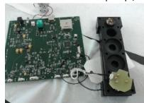
During the STM period, the attention has been focused on the realization of a gas sensing device. In detail, electrochemical sensors have been explored and the sensor calibration step has been studied in depth.
