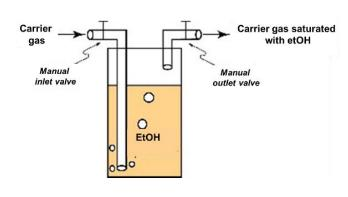
These are incorporated in bubbler, and one is longer than the other. The longer one allows the carrier gas to flow into bubbler favouring the dissolution of analyte and the its passage in the gaseous phase to form a saturated gas solution in the head space. Then, the forming gas bubbles can be moved away by the carrier gas through the shorter tube. The whole process is regulated by inlet and outlet valves and the sequence of opening/closing of which is very important.
