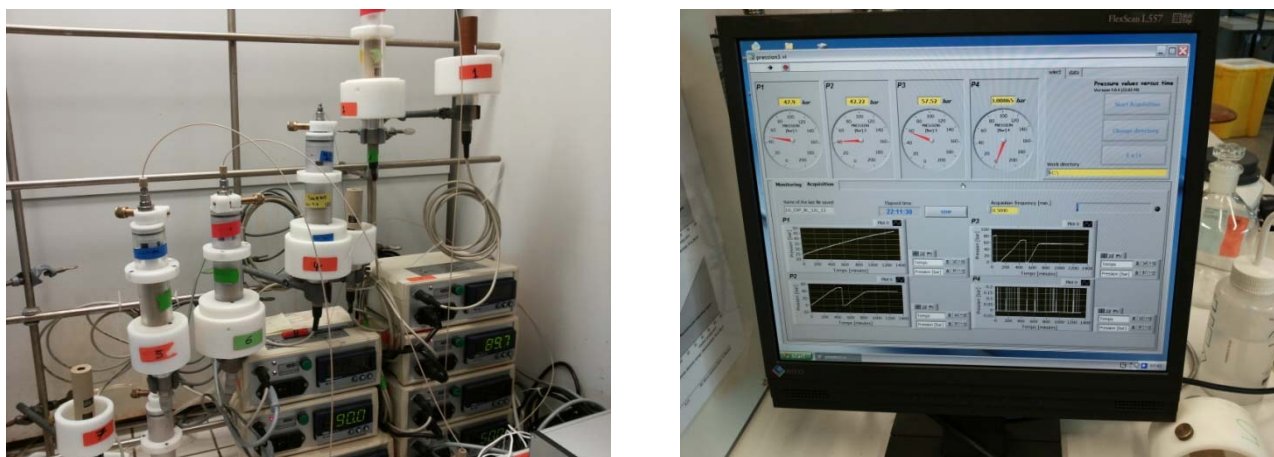
Figure 1 (left): A setup of four different FA dehydrogenation tests using HPNMR tubes; (right) pressure evolution monitoring by automated digital system.
