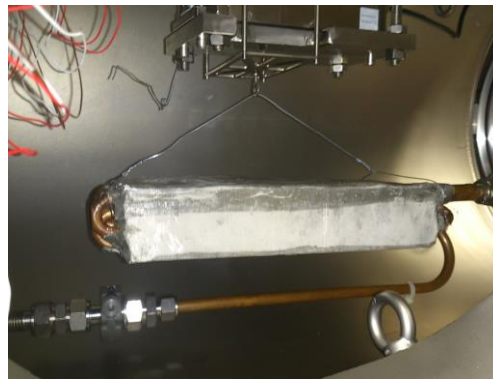
Figure 4 Granular AdHEX placed into the ISE kinetic set-up
