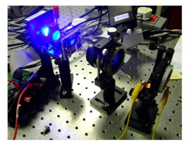
The LCD has been linearized both by the characterization of the wavefront acquired by the wavefront sensor and by a blue LED light intensity measurement. The figure below shows the sigmoidal modulation of the stroke of the deformable mirror in function of the blue gray level on the LCD. The function has been inverted to have a linear modulation necessary for the closed loop system.
