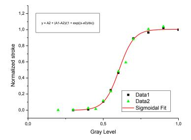
The measured DM stroke in function of the linearized gray level is reported in the graph below.
