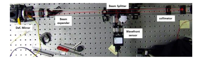
The PCDM is driven by a Liquid Crystal Display (LCD) 800x 600pixles which is illuminated with a high power blue LED. The LCD is imaged on the back of the PCD by the use of lens as illustrated in the figure and in the photo below.
