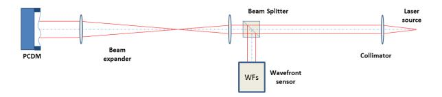
A photo of the apparatus mounted in Galway is in the next picture. The system is composed by a laser point source which is collimated and then expanded to match the active area of the PCDM which is of 10mm. In the second arm the beam reflected by the PCDM enters the a high resolution Shack-Hartmann wavefront sensor (f=6mm, pitch 200um) which has an optical aperture of 5mm.
