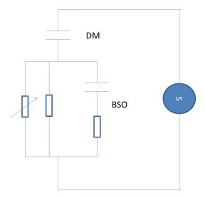
The membrane forms a capacitor  $C_{DM}$  while the Bismuth Silicon Oxide (BSO) crystal is modeled as a parallel between the BSO dark resistor  $R_{dark}$ , the photoconductor resistor  $R_{PH}$  and the series between a capacitor  $C_{BSO}$  and a resistor  $R_{BSO}$ .
