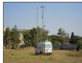
Fig.2 Mobile Laboratory and 2 stations very close each other for eddy correlation measurement.
