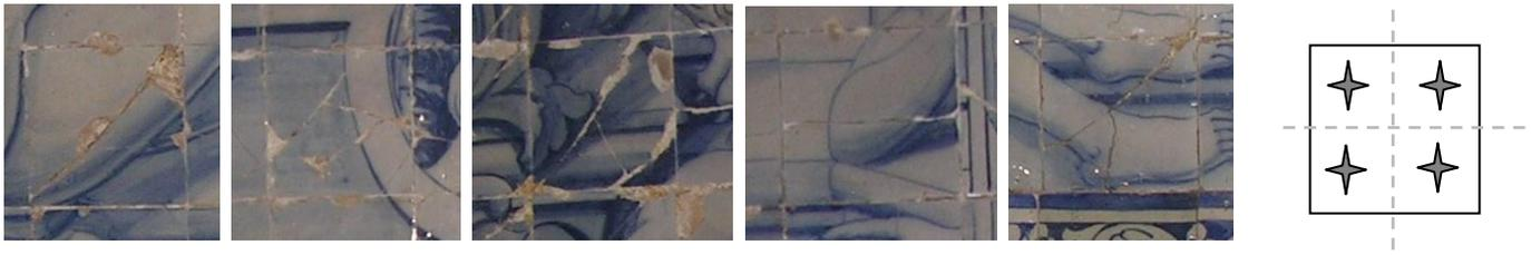
**Fig.10:** Fracture profiles in single tiles, and acquisition points arrangement for single tile.
