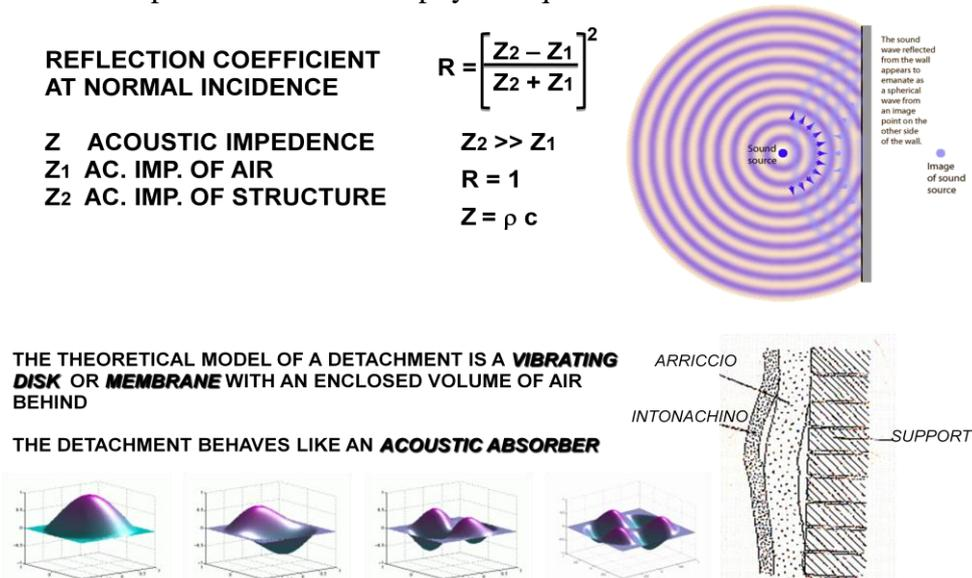
**Fig.4:** Scheme of the interaction between acoustic wave and the structure under study.
