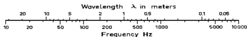
**Fig.13:** Wavelength to frequency conversion for the speed of sound in air of 343 m/sec.
