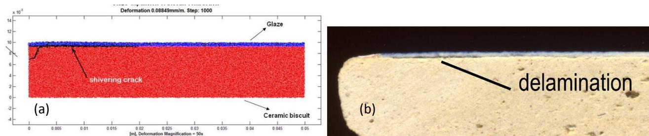
**Fig.2:** Delamination between clay bisque and glaze, (a) numerical model and (b) real sample.
