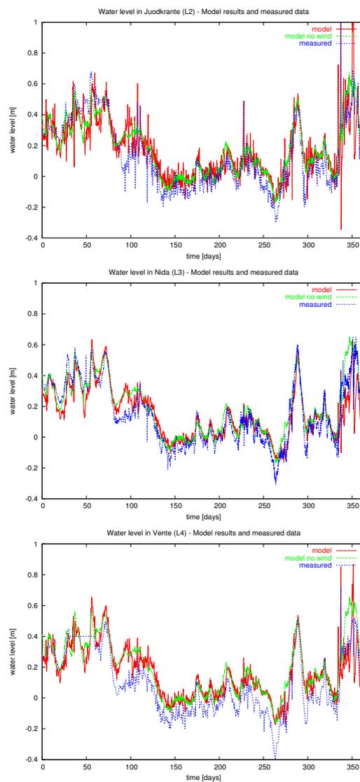
Figure 9. Water level: numerical results and experimental data in 3 station inside the lagoon [year 1999].
