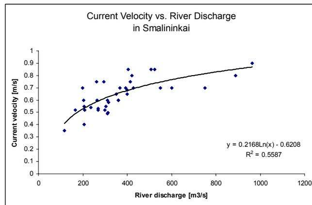
Figure 4. Relation between the current velocity and the river discharge in Smalininkai. The water arrived to the Nemunas delta with a delay respect to Smalininkai which depend on the velocity, and then to the discharge.
