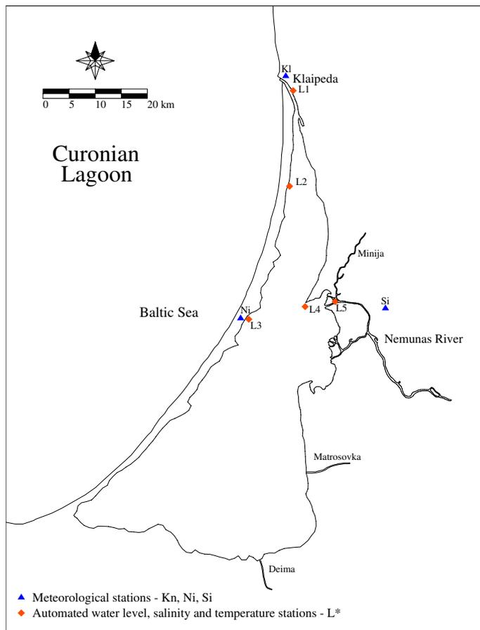
Figure 3. Data station used as input in the model:  $L^*$  = water level stations,  $Km^*$  = current velocity and direction, salinity and water temperature stations,  $Kl$  and  $Ni$  = meteorological stations.
