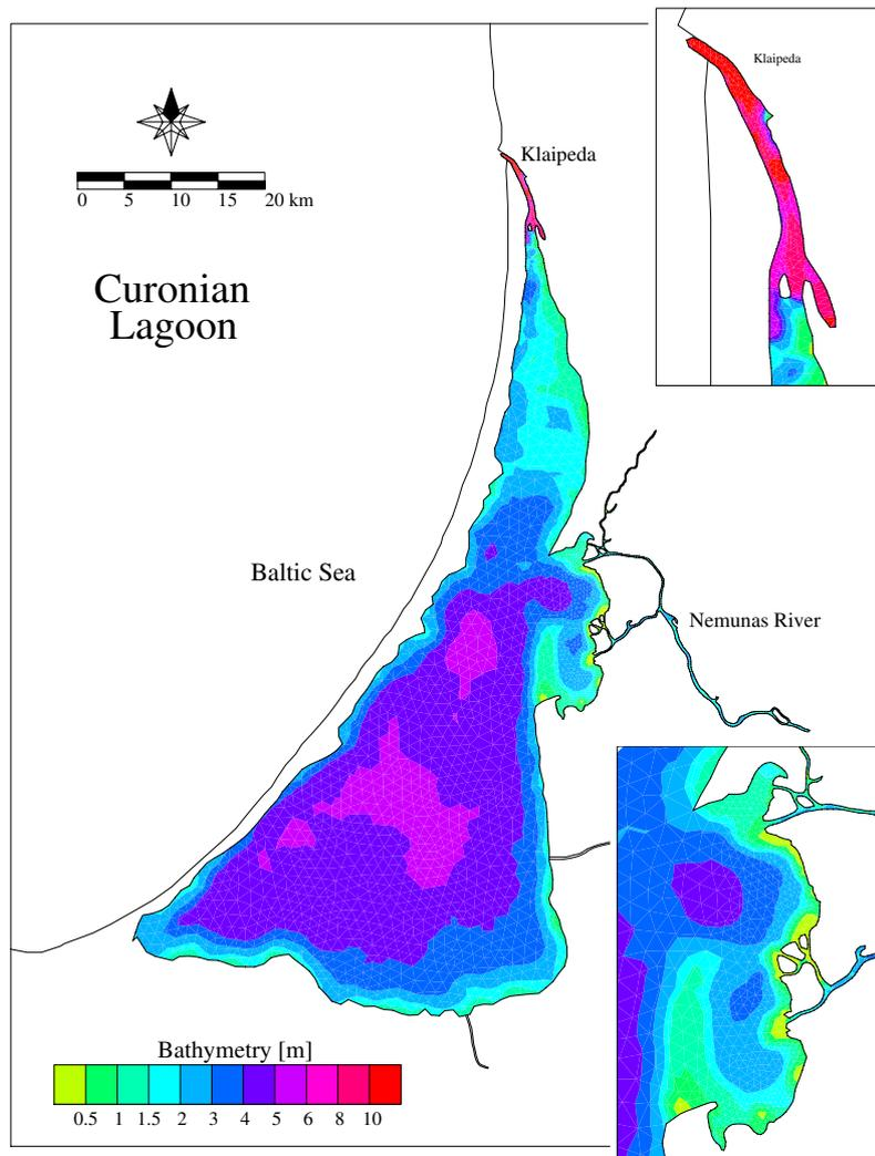
Figure 2. Bathymetry of the Curonian Lagoon as computed by the model.
