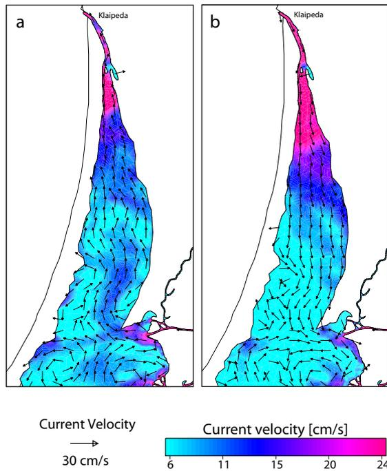
Figure 7. Water current field in the northern part of the Curonian lagoon. a) outgoing flow (situation with high Nemunas discharge), b) ingoing flow (situation with strong north wind).
