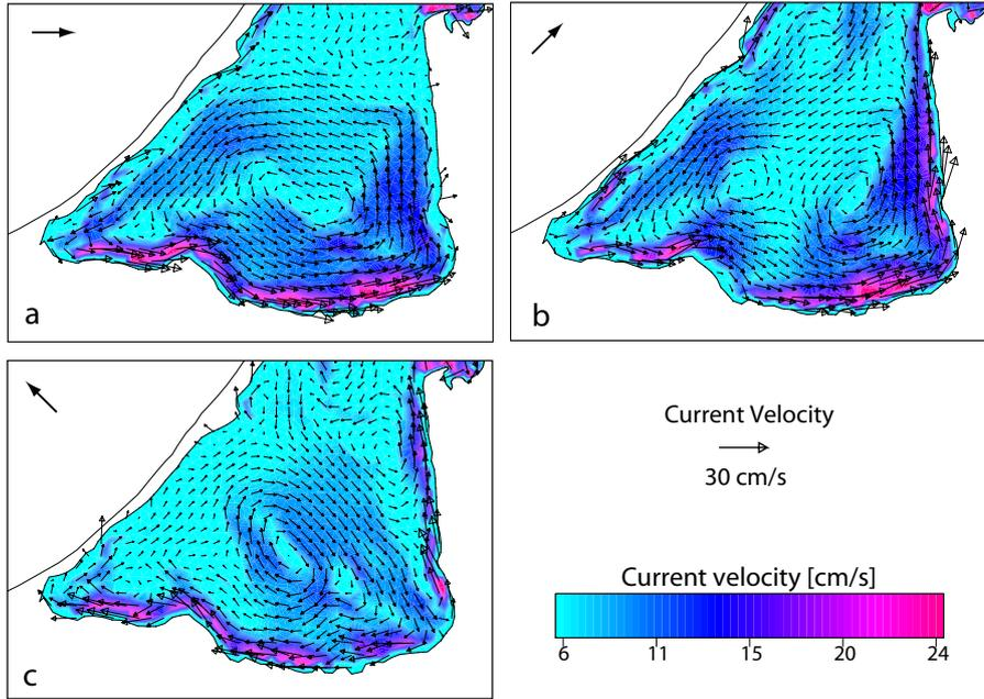
Figure 6. Wind driven circulation in the southern part of the Curonian lagoon. a) west wind, b) south-west wind, c) south-east wind [wind intensity = 10 m/s].
