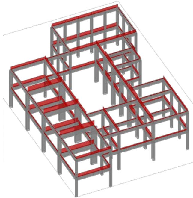
Fig. C-10 Preliminary model and load distribution from the floors on the beams.
