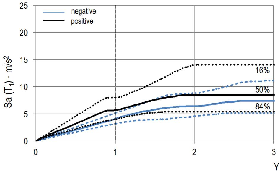
Fig. B-40 ISA curves obtained by comparing the median capacity curve and the median response spectrum (at the 16% and 84% percentiles): Amm-1, X-direction (positive and negative direction) and SLD.
