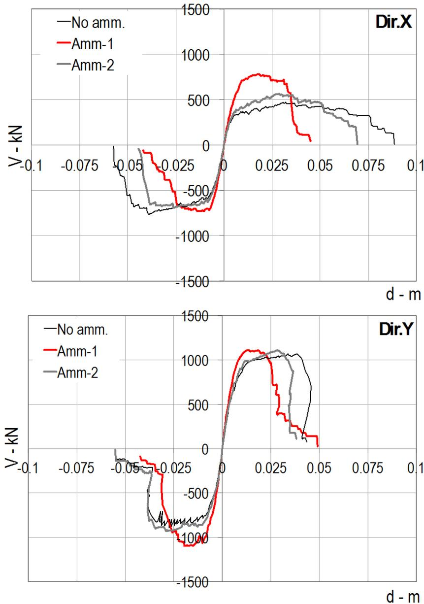
Fig. B-13 The resulting pushover curves in X and Y direction (positive and negative) as a function of the three hypotheses assessed for the wall-to-wall connection (Amm-1, Amm-2 and absence of connection)
