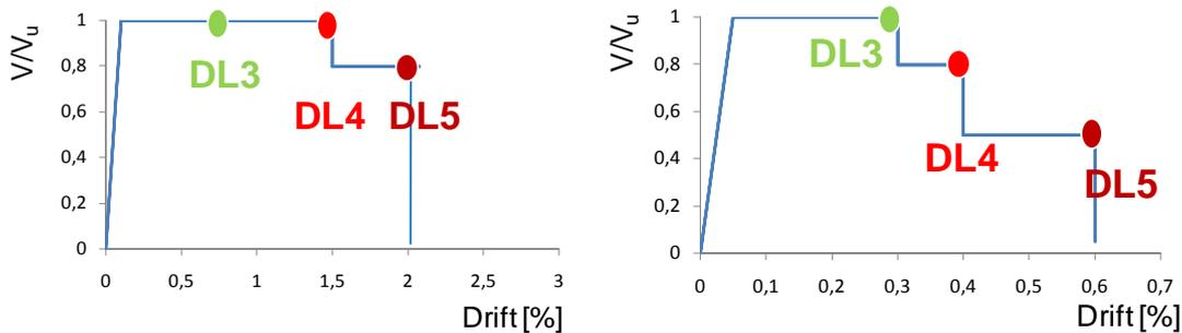
Fig. 3-3. Constitutive shear-drift laws for masonry piers: failure under normal force and bending (left) and shear failure (right).
