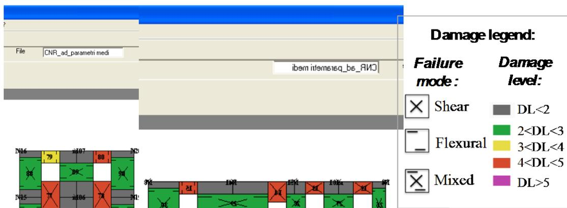
Fig. B-21 Damage simulated for the walls 4 and 1 oriented in the X direction
