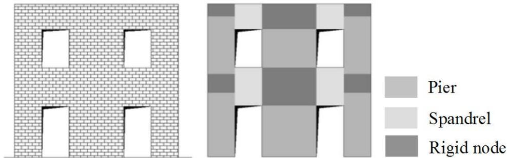
Fig. 3-1 Idealization of a masonry wall into the equivalent frame
