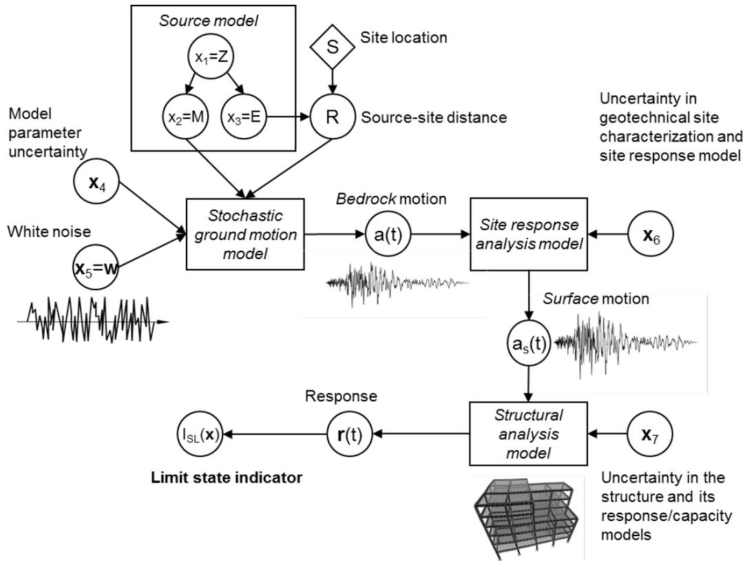
Fig. A-1 Diagram of simulation procedure with reference to generic event.
