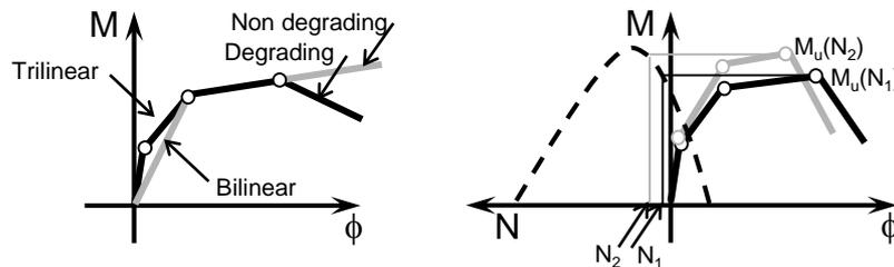
Fig. 4-3 Direct section models: alternatives for the monotonic curve (left), effect of the interaction between the normal force and bending moment (right).
