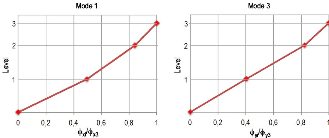
Fig. B-23 Deformed shape in height of the modes 1 and 3 for model Amm-1 (first branch of the logic tree).
