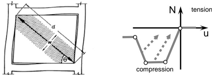
Fig. 4-7 Equivalent strut for a panel (left), and typical cyclic law (left).
