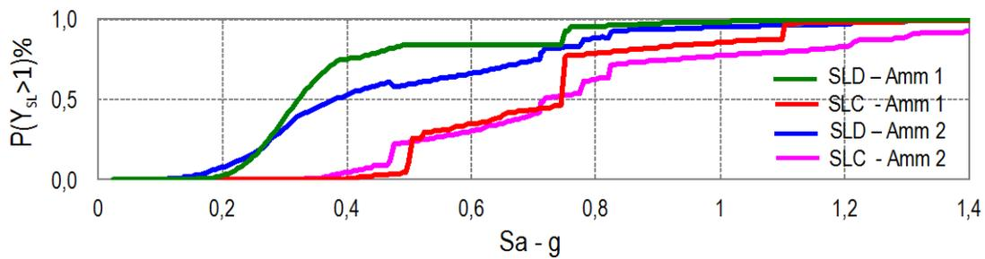
Fig. B-50 Fragility curves for the three limit states, obtained by the two branches of the logic tree.
