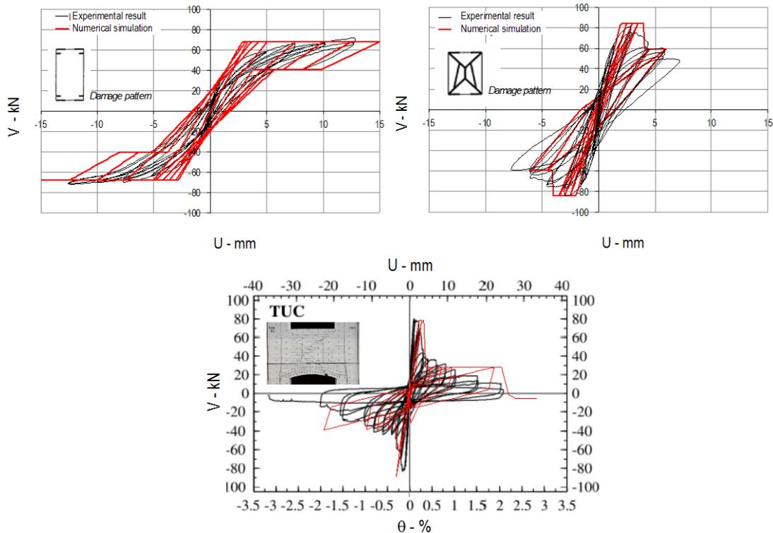
Fig. B -10 Numerical simulation of some panels tested in laboratory, aimed at calibrating the hysteretic parameters of the piecewise-linear model adopted (in the case of piers reference was made to the experimental results of Anthoine et al. 1995, in the case of spandrels to those of Beyer and Dazio, 2012)
