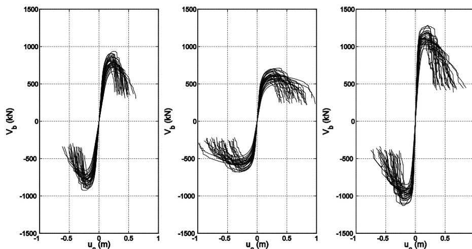
Fig. C-21 Model A: Dispersion in the capacity curves for the three significant modes.
