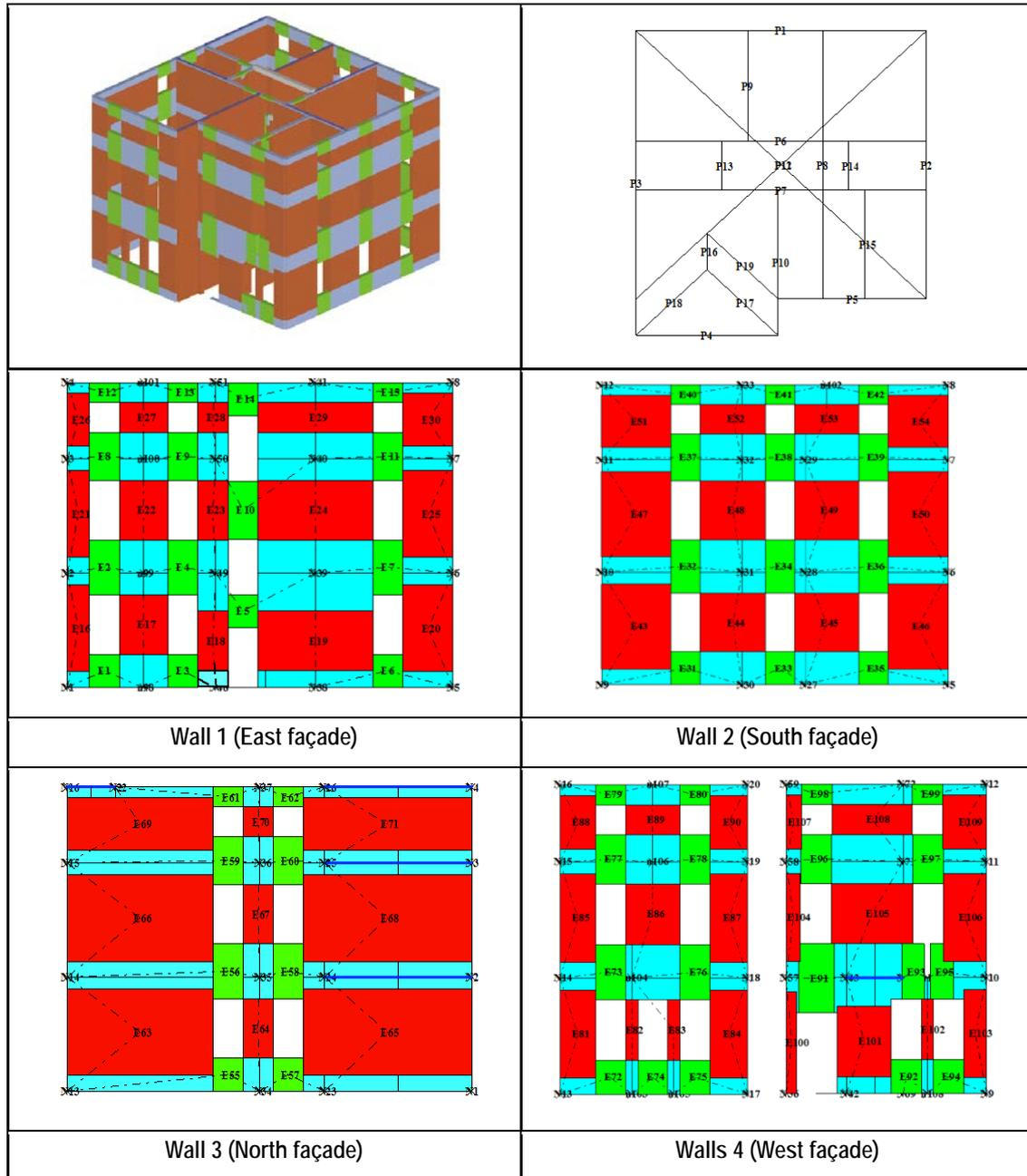
Fig. B -8 Three-dimensional structural model, numbering plan of the walls and a possible equivalent frame idealization of the main façades (the dotted lines graphically identify the position of the center of gravity of the structural element with respect to the end nodes which it is attached to)
