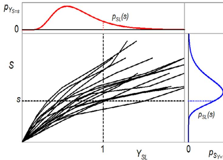
Fig. A-2 Evaluation of fragility starting from the IDA curves using Eqs. (2.14) and (A.8).
