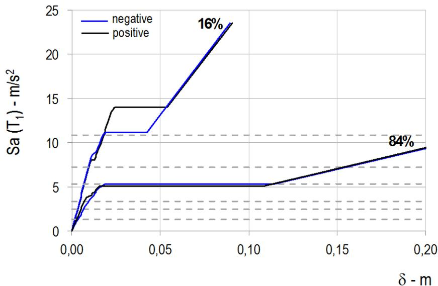
Fig. B-47 ISA Curves calculated by comparing the median capacity curve with the response spectra at 16% and 84% percentiles
