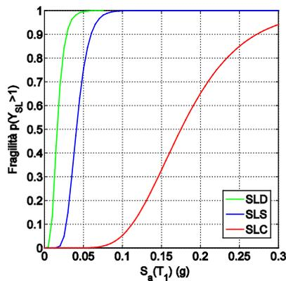
Fig. C-25 Model A: Fragility curves for the three limit states.
