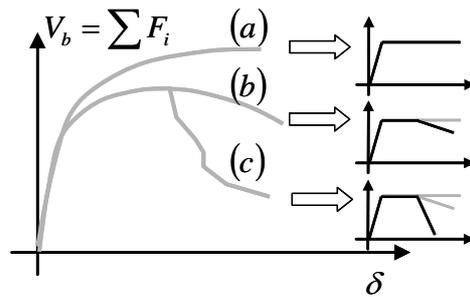
Fig. 2-5 Effect of modelling on the relationship between base shear and top displacement, and qualitative laws of the equivalent oscillator.
