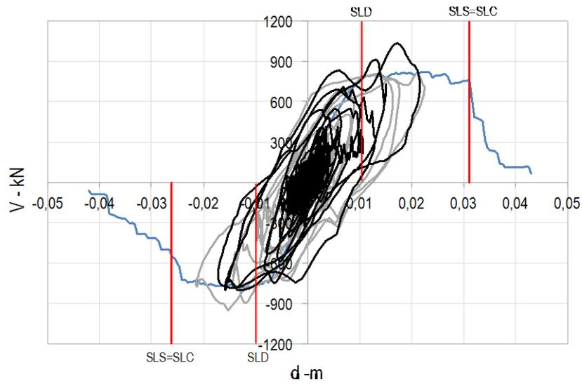
Fig. B-19 Direction X: comparison of the results of non-linear static and dynamic analysis
