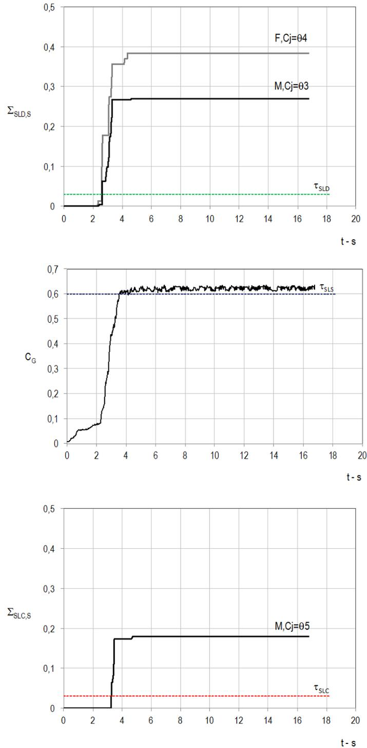
Fig. B-27 Variation with time of the entities necessary for the calculation of the limit state variables at the scale of the element (the cumulative damage indicators  $\Sigma_{SLD}$ ,  $\Sigma_{SLC}$ ) and cost function ( $C_G$ ), resulting from the application of the event 1 scaled to the value  $S_a(T_1) = 10.84 \text{ m/s}^2$ .
