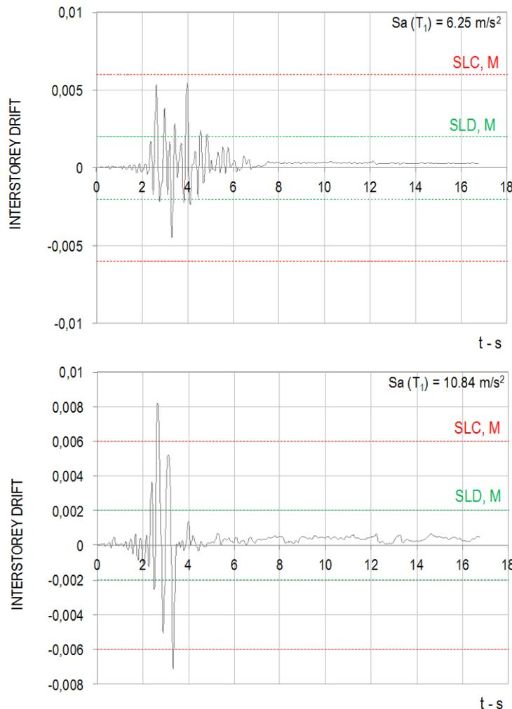
Fig. B-28 Variation with time of the interstorey drift, relatively to the wall and diaphragm that present the maximum values, for the two levels of the intensity measure shown in the previous Figures.
