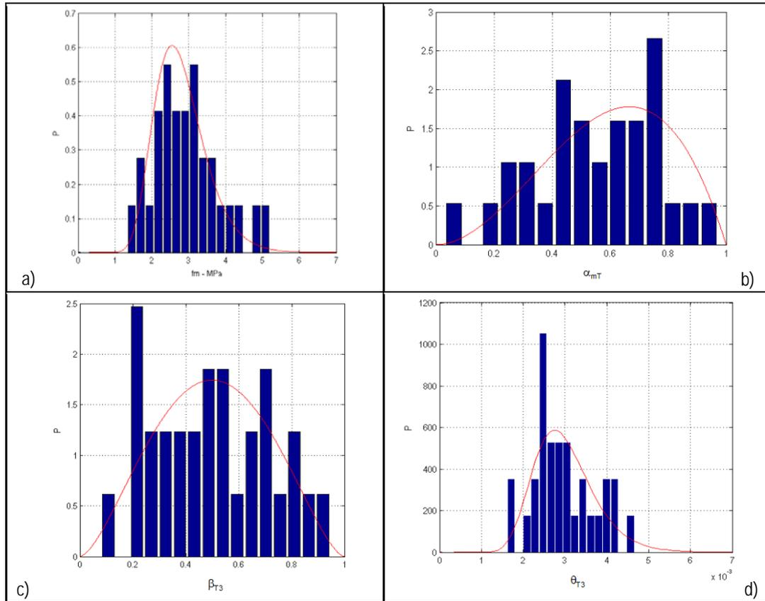
Fig. B-16 Histograms relating to the distribution of the stochastic sampling obtained for some of the variables belonging to four of the sets of random variables considered: a) the compressive strength of the masonry  $f_m$  (from set 1 - Masonry); b)  $\alpha_{mT}$  (from set 8 - Energy dissipation of piers); c)  $\beta_{T3}$  (from set 7 - constitutive law of spandrels);  $\theta_{T3}$  (from set 6 - constitutive law of piers).
