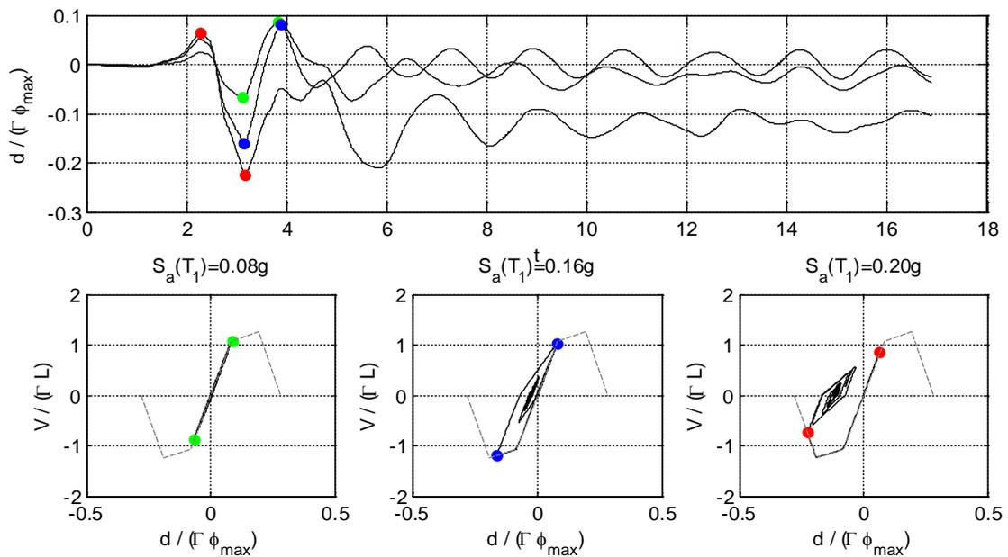
Fig. C-33 Example of cyclic degrading response of the equivalent oscillator (structure and signal n° 1): time histories of the displacement response for three different intensities (top), the force-deflection cycles for the lower intensity (below, left), average (below, center) and for the higher intensity (down, right).
