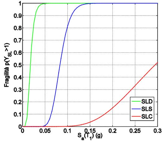
Fig. C-31 Model C: Fragility curves for the three SL.
