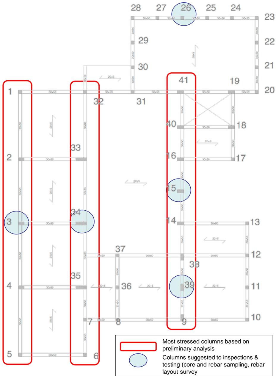
Fig. C-11 Position of the elements subject to testing.
