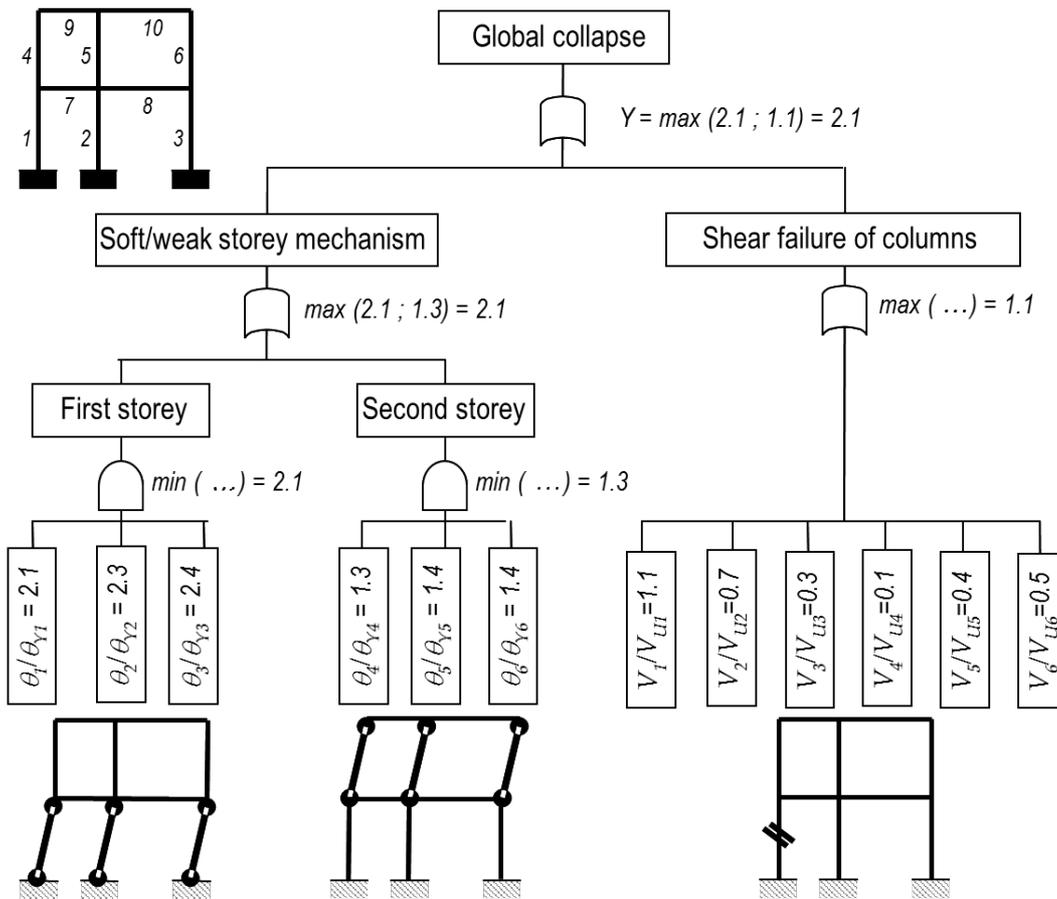
Fig. A-8 Representation of structural failure as a combination of alternative sub-systems (mechanisms).
