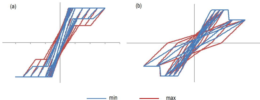
Fig. B-15 Effect of the parameters  $\alpha_m$ ,  $\gamma_m$  and  $\delta_m$  on the hysteretic response at scale of the single masonry panel: a pier with a prevailing flexural (a) or shear (b) response
