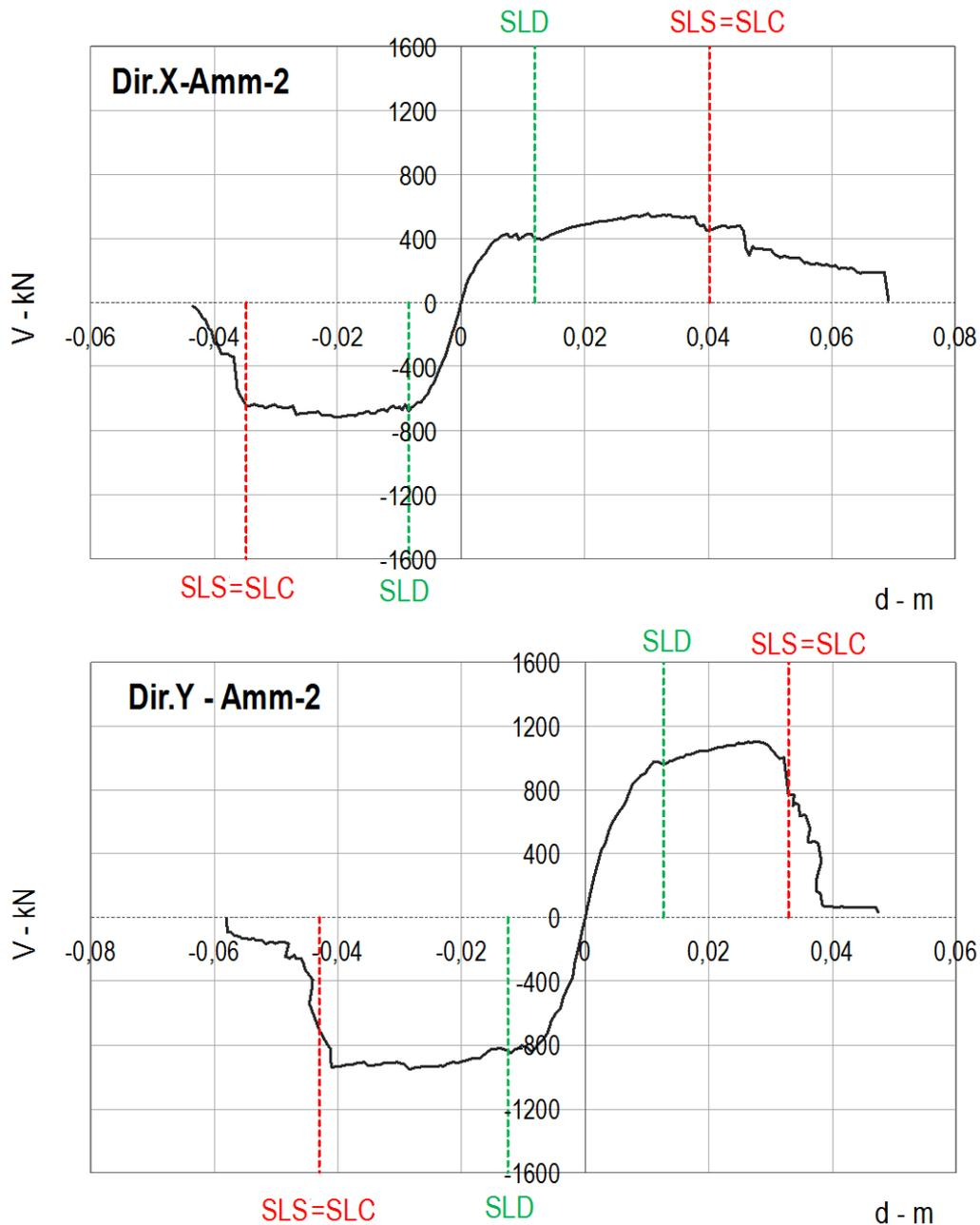
Fig. B-34 Results of the non-linear static analyses for the second branch of the logic tree (Amm-2) in the directions X and Y, with positive and negative direction (mean values for all the random variables)
