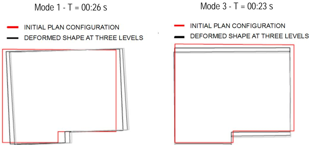
Fig. B-22 Plan deformed shape related to the modes 1 and 3 for model Amm-1 (first branch of the logic tree); the different colors are associated with the different levels of the building.
