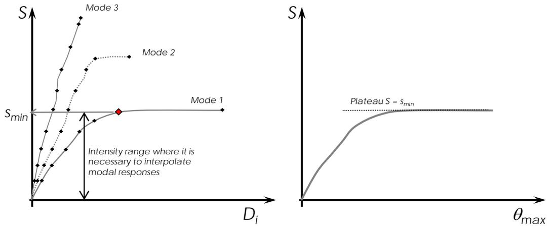
Fig. C -16 The IDA curves of the modes (left) and that of the entire structure (right).
