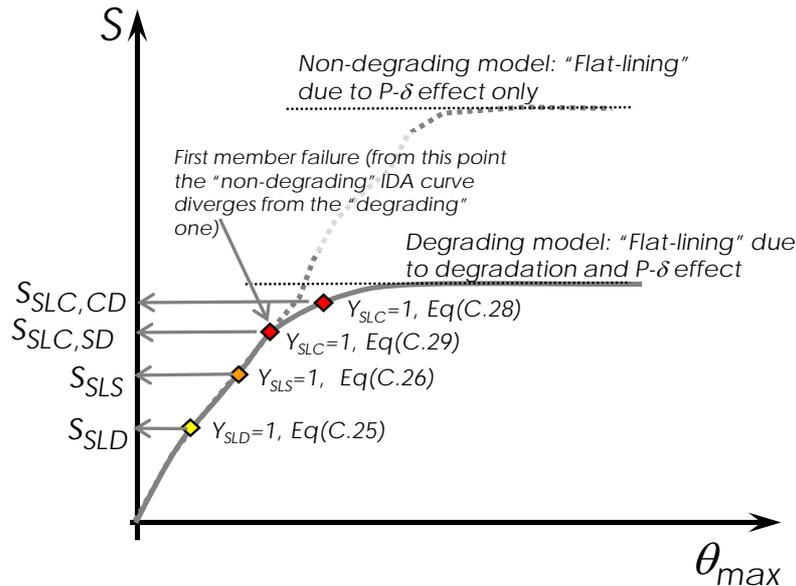
Fig. C -17 The IDA curve of the entire structure and representation of the attainment of the three SLs, for the two types of modelling considered.
