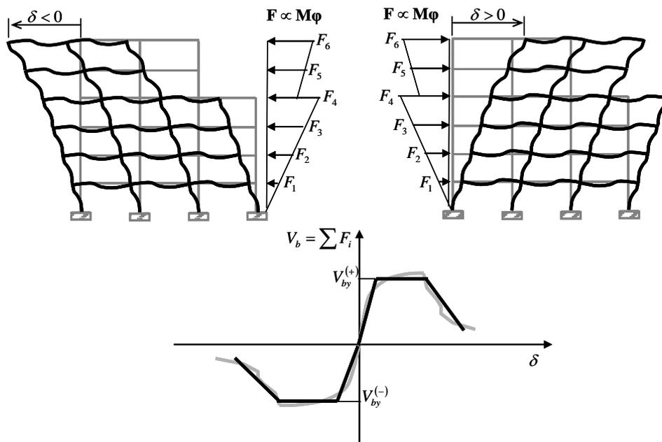
Fig. 2-4 Determination of the monotonic envelope of the constitutive relationship of the equivalent oscillator in the case of non-symmetrical behaviour and modelling with laws characterized by degradation.
