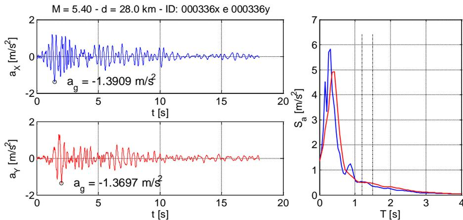
Fig. C-8 Record No. 3: time histories of the orthogonal components of horizontal acceleration, and respective response spectra.
