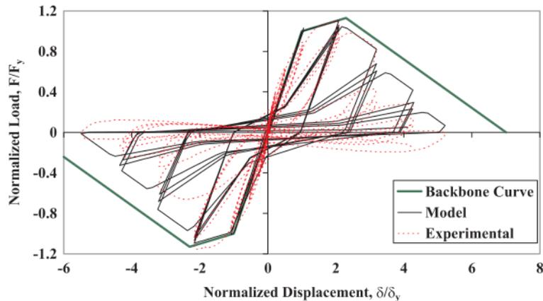
Fig. 4-6 Experimental cyclic response of a reinforced concrete column built according to old concepts and numerical simulation (adapted by Ibarra et al 2005).
