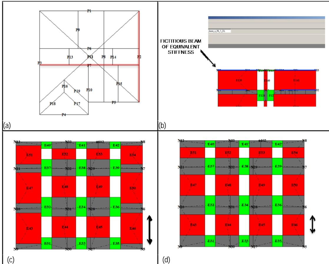
Fig. B -11. Equivalent frame model (piers in red, spandrels in green, rigid nodes in grey): (a) plan view of masonry walls; (b) internal wall 7 in which the fictitious beams adopted for simulating the flange effect are indicated; (c/d) exemplification of the two assumptions adopted for the geometry of piers, by way of example in the case of wall 2: (c) Mesh-1 and (d) Mesh-2.
