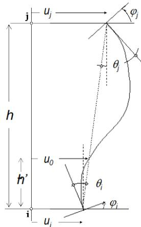
Fig. 3-2. Definition of the terms useful for the calculation of the drift according to (3.10)
