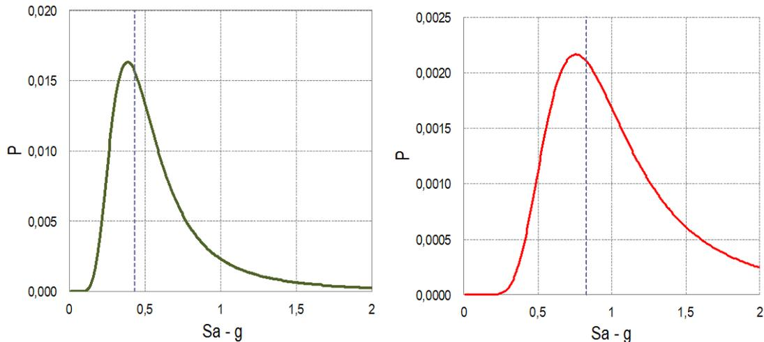
Fig. B-32 Distribution of the conditional probability for the computation of the limit states SLD and SLC (the vertical dotted line indicates the median value of the seismic intensity measure which leads to the attainment of SL).
