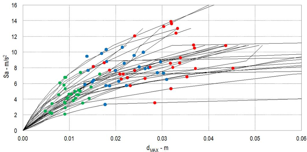
Fig. B-29 Incremental Dynamic Analysis (IDA) curves in terms of maximum displacement at the top of the building versus the seismic intensity measure, for the 30 models considered; the green, blue and red dots correspond to the achievement of the SLD, SLS and SLC, respectively.
