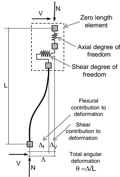
Fig. 4-5 Model consisting of a bending element and of elements at zero length for the shear, the axial failure and the sliding of the bars.
