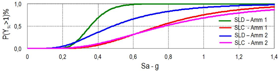
Fig. B-44 Fragility curves for the three limit states, obtained by the two branches of the logic tree.
