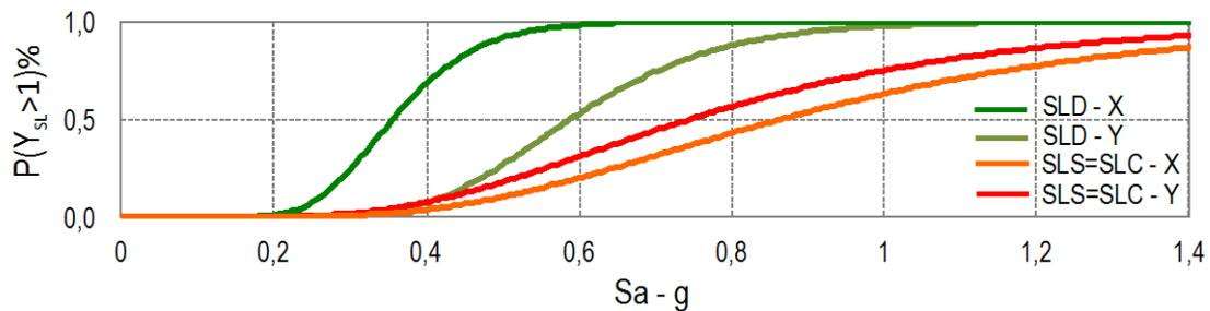
Fig. B-42 Fragility curves for the three limit states, obtained for the first branch of the logic tree, considering the response in the two X and Y directions.
