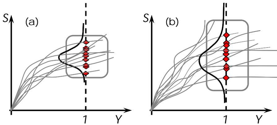
Fig. 2-6 IDA Curves: (a) without randomness of the structure (b) with randomness of the structure.
