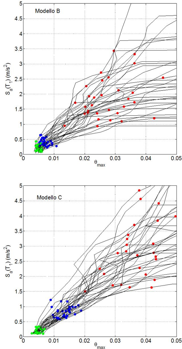
Fig. C-28 Models B (above) and C (below): IDA curves of the structure (combination of modal curves, see Fig. C-16).
