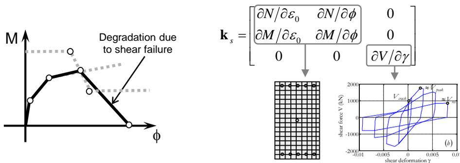
Fig. 4-4 Direct sectional models: alternatives for the monotonic curve (left), effect of the interaction between the stresses (right).
