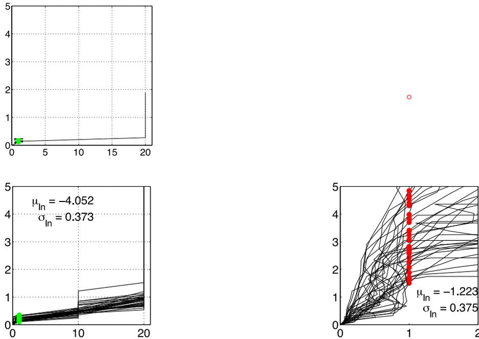
Fig. C-29 Models B (above) and C (below): Details of IDA curves in terms of the limit state variables.
