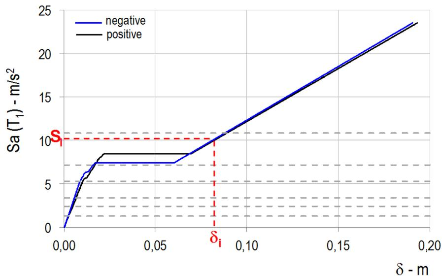
Fig. B-46 ISA curves obtained from the comparison between the median capacity curve and the median response spectrum as a function of the positive and negative directions (X direction -Amm.1): the horizontal dotted lines exemplify the potential use of such curves for 6 different values of the seismic intensity as shown in Table B-18.
