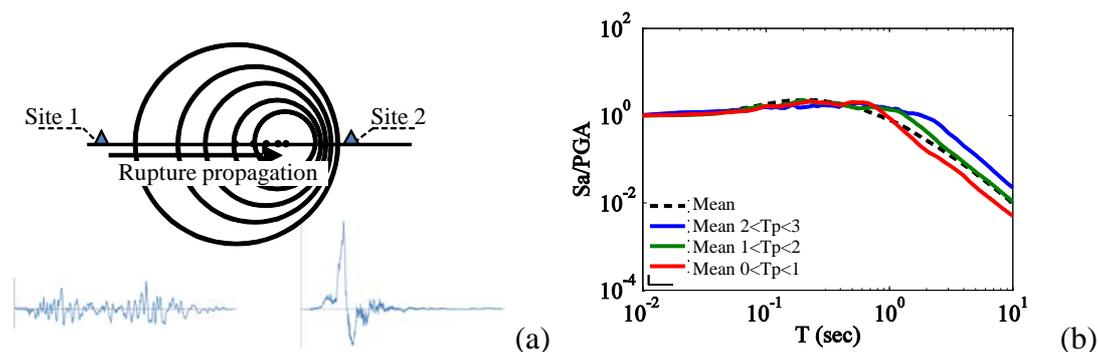
Fig. A-7 (a) Simplified illustration of the impulsive effects of directionality and example relating to the Landers earthquake, California (1992). (b) Mean elastic acceleration spectra in the case of impulsive and ordinary signals; all of the spectra are normalized to the same PGA values. Note the systematic difference around the pulse period.
