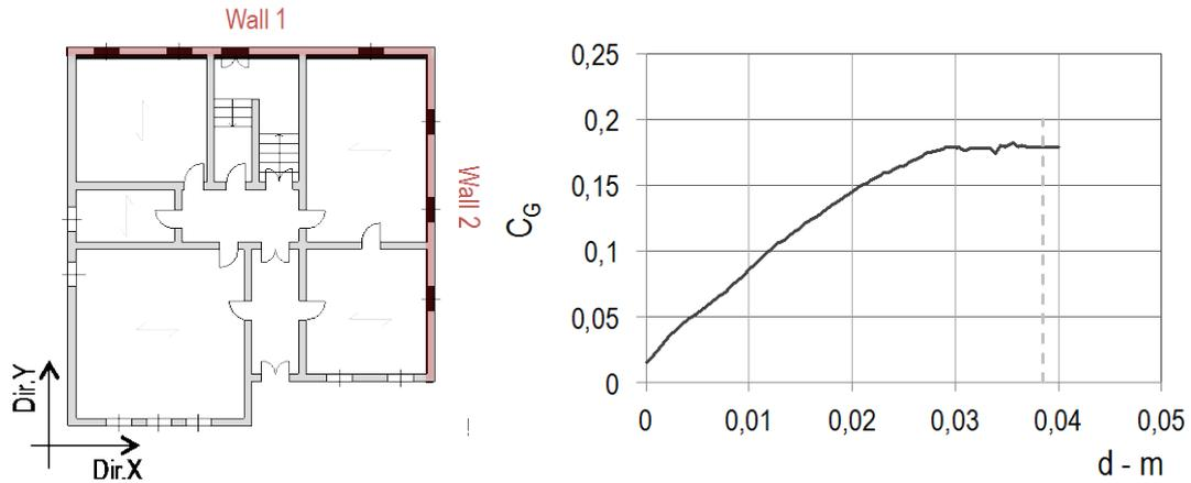
Fig. B-36 a) Identification in plan of the walls 1 and 2; b) cost function resulting from the non-linear analysis in X- positive direction.
