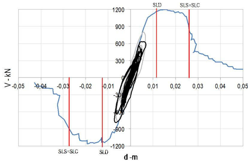
Fig. B-20 Direction Y: comparison between the results of non-linear static and dynamic analyses
