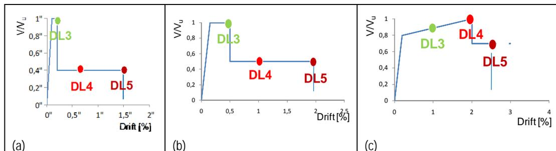
Fig. 3-4. Constitutive drift-shear laws for spandrels supported by: a) a masonry arch; b) a lintel in timber, steel or reinforced concrete; c) a lintel coupled to a tensile-resistant element.
