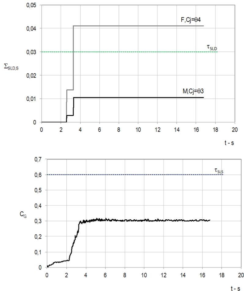
Fig. B-26 Variation with time of the entities necessary for the calculation of the limit state variables at the scale of the element (the cumulative damage indicator  $\Sigma_{SLD}$ ) and the cost function ( $C_G$ ), resulting from the application of the event 1 scaled to the value  $S_a(T_1) = 6.25 \text{ m/s}^2$ .
