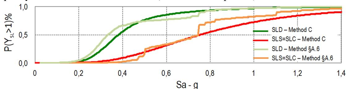
Fig. B-52 Final fragility curves for the three limit states compared as obtained by the method C and method illustrated in §A.1.1.1. (as resulting from the combination of two branches of the logic tree)
