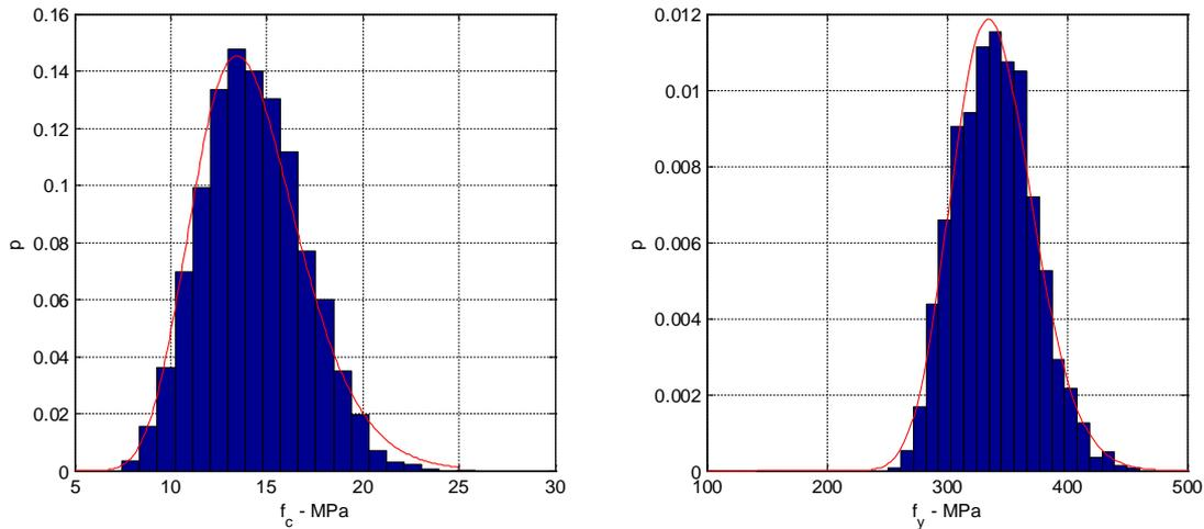
Fig. C -13 Properties of the materials: histograms of the relative frequency of sampled values and corresponding density (histograms are obtained with all the sampled values, i.e. for all elements in all the N simulations).
