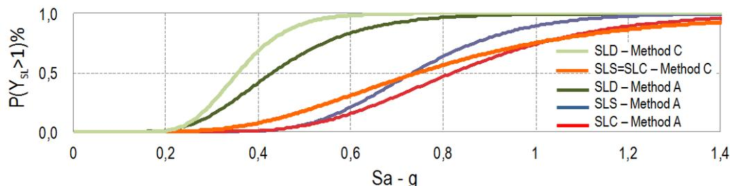
Fig. B-53 Final fragility curves for the three limit states, obtained by combining the results of the two branches of the logic tree (Amm-1 and Amm-2).
