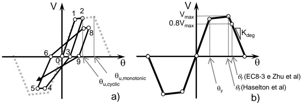
Fig. 4-9 (a) Monotonic threshold (model with degradation) and cyclic threshold (model without degradation) (b) definition of different thresholds for the start of the negative stiffness.
