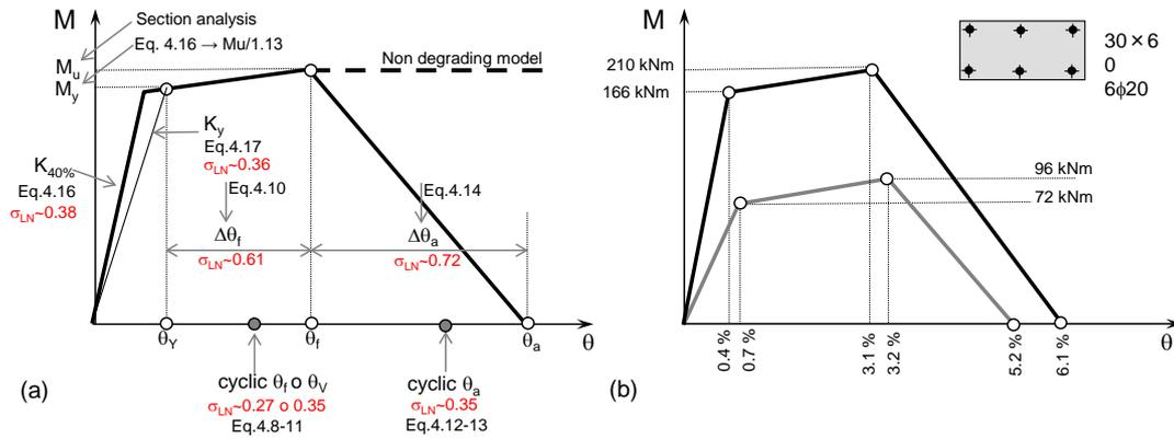
Fig. C -18 Constitutive law of plastic hinge (a) and laws in the two planes of bending for a rectangular column (b).
