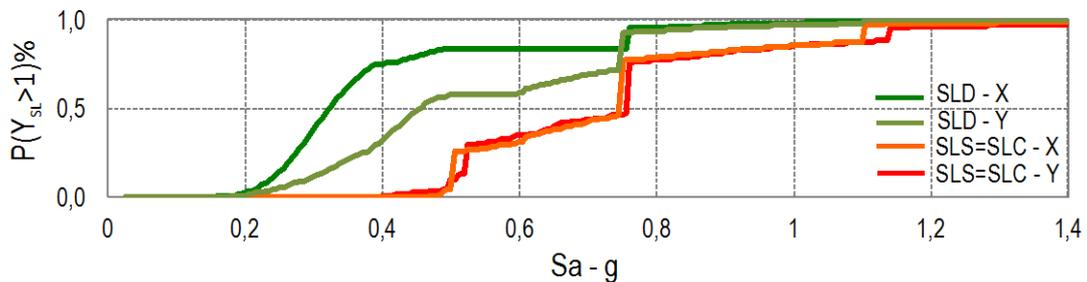
Fig. B-48 Fragility curves for the three limit states, obtained for the first branch of the logic tree, considering the response in the two directions X and Y according to the approach proposed in Appendix A.1.1.1..
