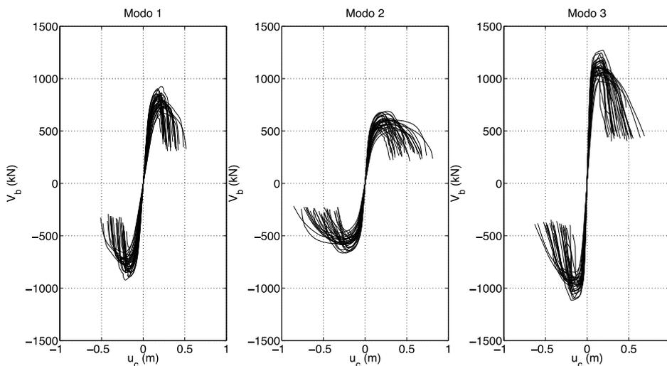
Fig. C-26 Model B: Dispersion in capacity curves for the three significant modes.
