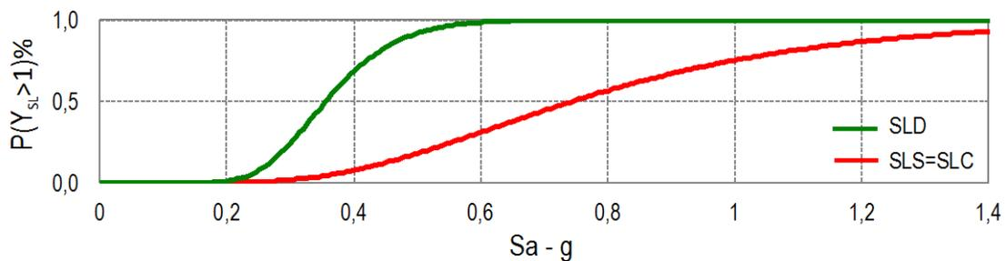
Fig. B-43 Fragility curves for the three limit states, obtained for the first branch of the logic tree (Amm-1).
