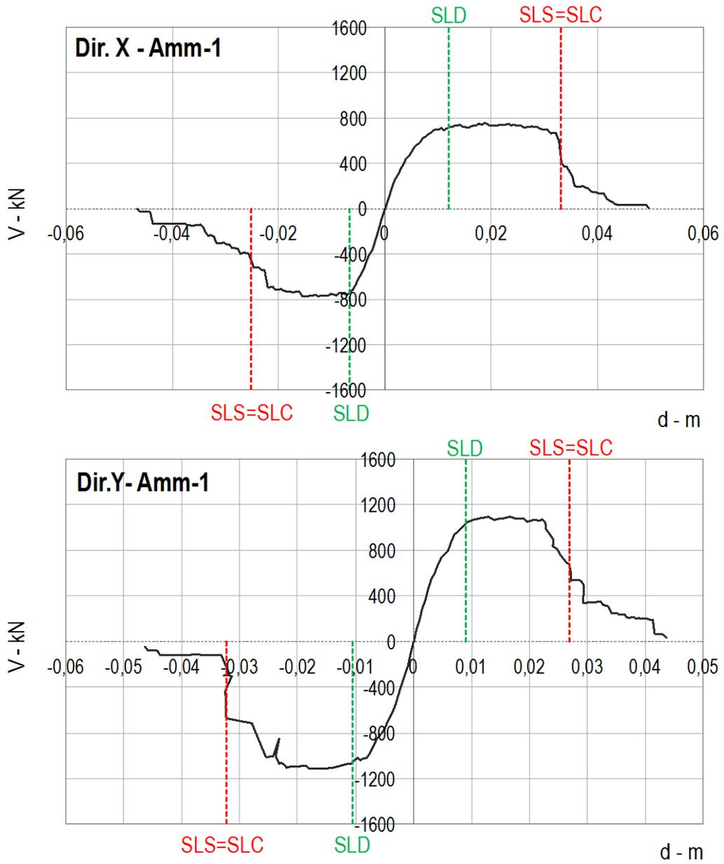
Fig. B-33 Results of the non-linear static analyses for the first branch of the logic tree (Amm-1) in the direction X and Y, with positive and negative direction (mean values for all the random variables)
