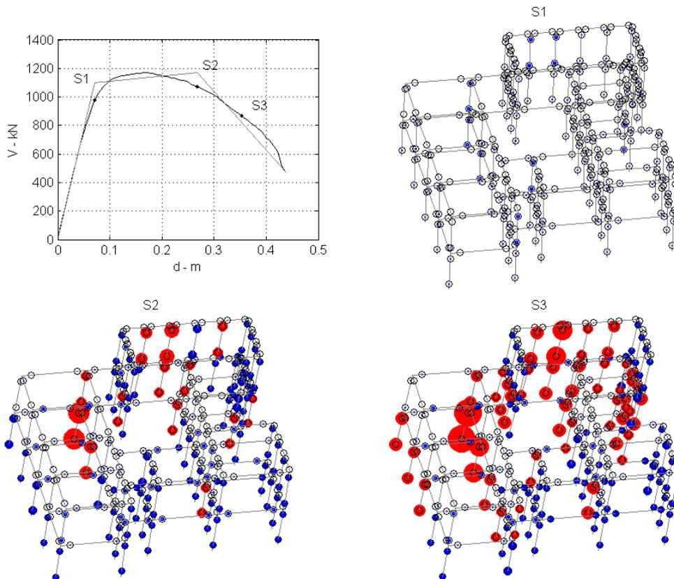
Fig. C-32 Capacity curve and deformations corresponding to the three points: yield strength, peak and intermediate on the branch of degradation.
