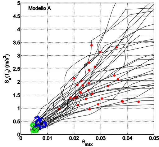
Fig. C-23 Model A: IDA curves of the structure (combination of the modal curves, see Fig. C-16).
