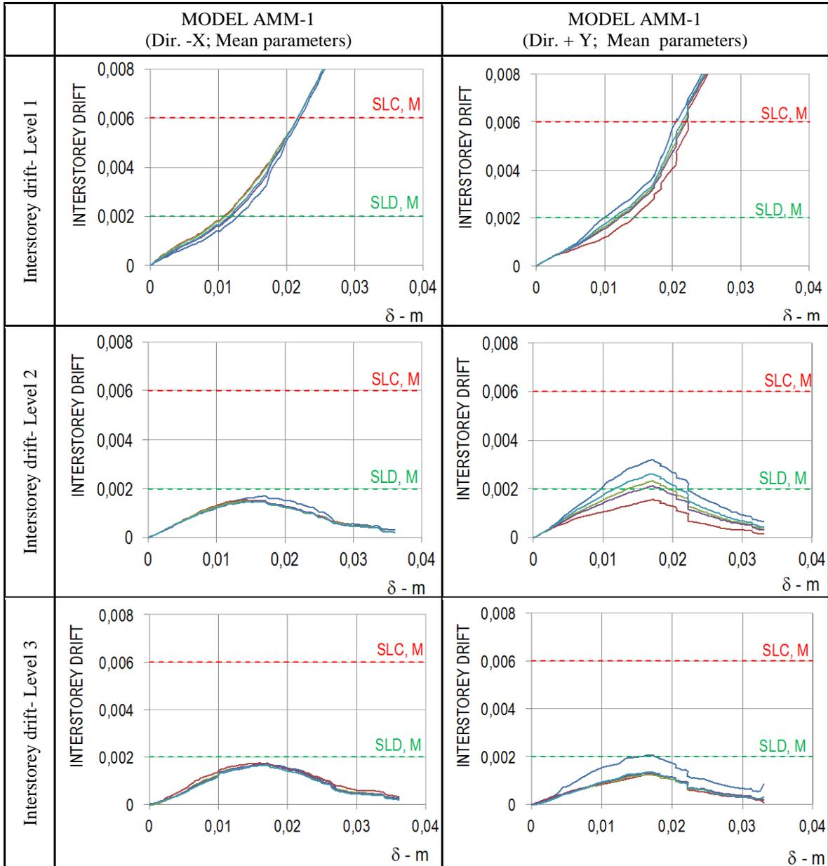
Fig. B-39 Evolution of the interstorey drift, at different levels of the building.
