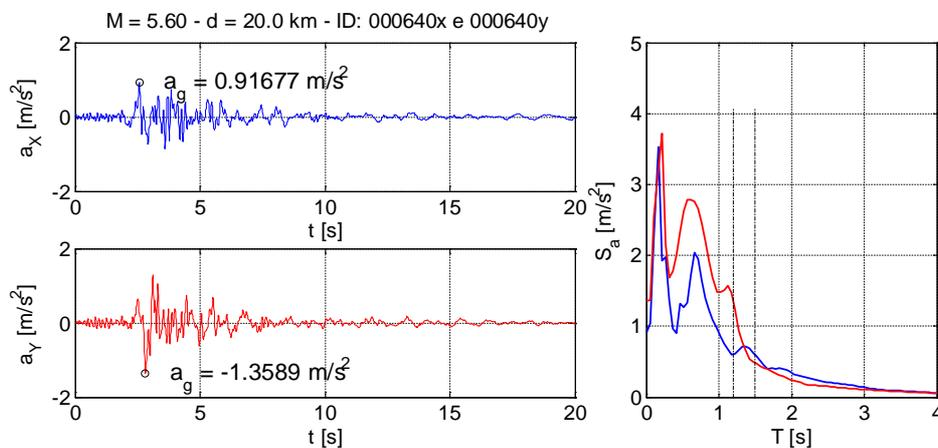
Fig. C-9 Record No. 4: time histories of the orthogonal components of horizontal acceleration, and respective response spectra.
