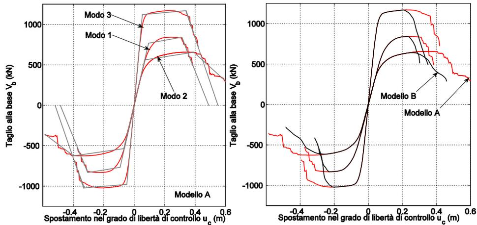
Fig. C -15 Capacity curve: trilinear approximation for the model A, without degradation, to the left, and comparison between model A and model B with degradation, right. The negative tangent in the model without degradation is due to the geometric contribution to the stiffness.
