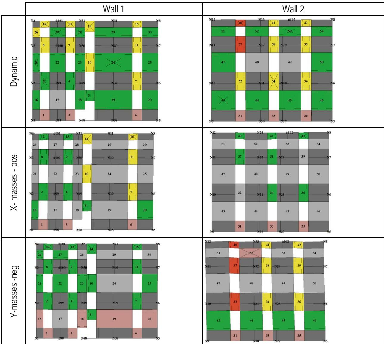
Fig. B-37 Comparison between the damage of the walls 1 and 2 obtained at the end of the non-linear dynamic analysis (event 1 scaled to the value  $S_a(T_i) = 6.25 \text{ m/s}^2$ ) and that resulting from the non-linear static analysis (X- positive direction and Y- negative direction) in correspondence of the step in which the maximum displacement obtained from the dynamic analysis is attained
