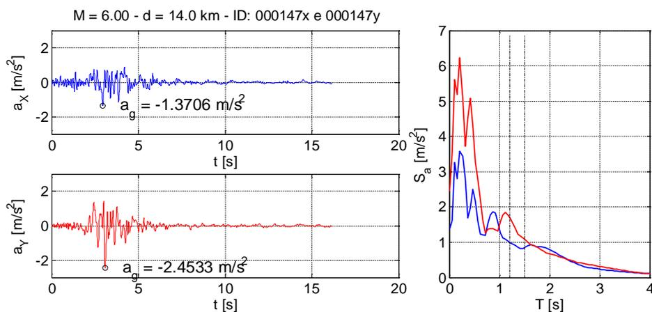
Fig. C-7 Record No. 1: time histories of the orthogonal components of horizontal acceleration, and respective response spectra (the two vertical lines indicate the range of variation of the fundamental periods of the 30 realizations of the models A or B).
