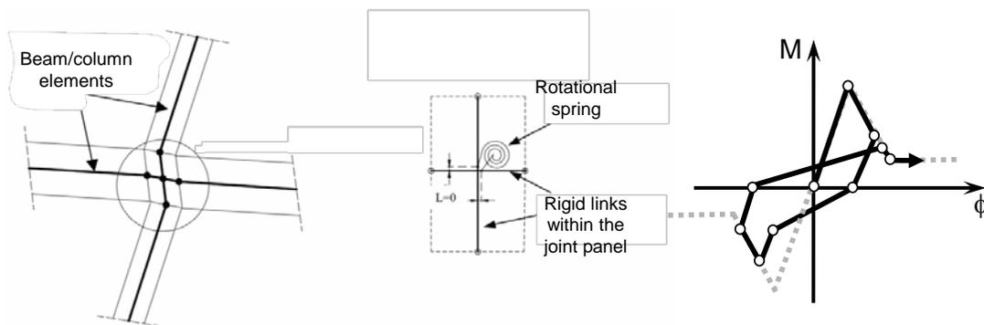
Fig 4-7 Response model for internal nodes: geometry (left), constitutive law (right)
