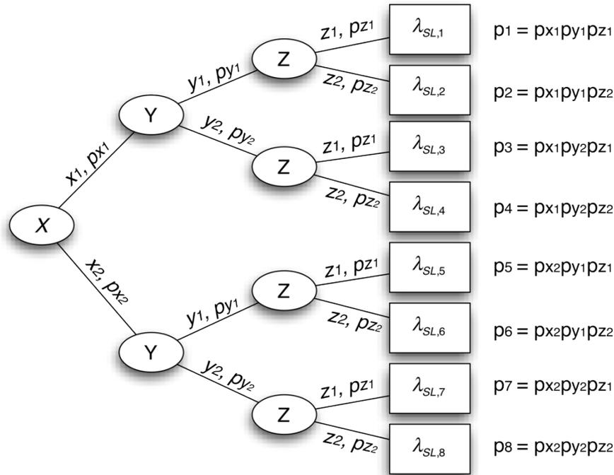
Fig. 2-2 Logic tree for three variables X, Y and Z each with two values.
