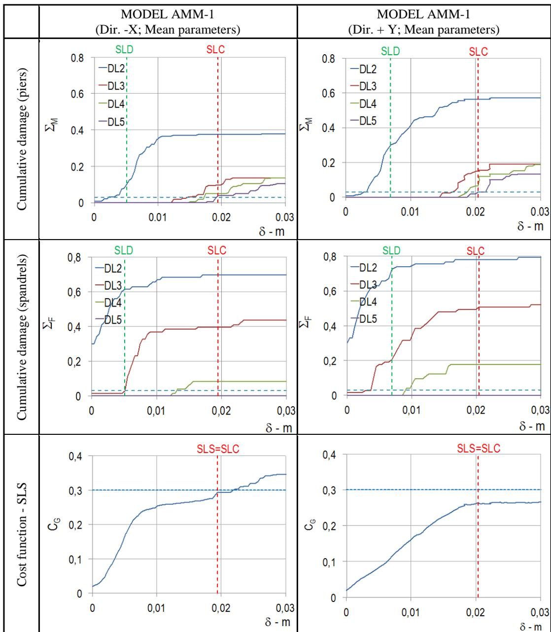
Fig. B-38 Evolution of the cumulative damage indicators of piers and spandrels and the global repair cost variable
