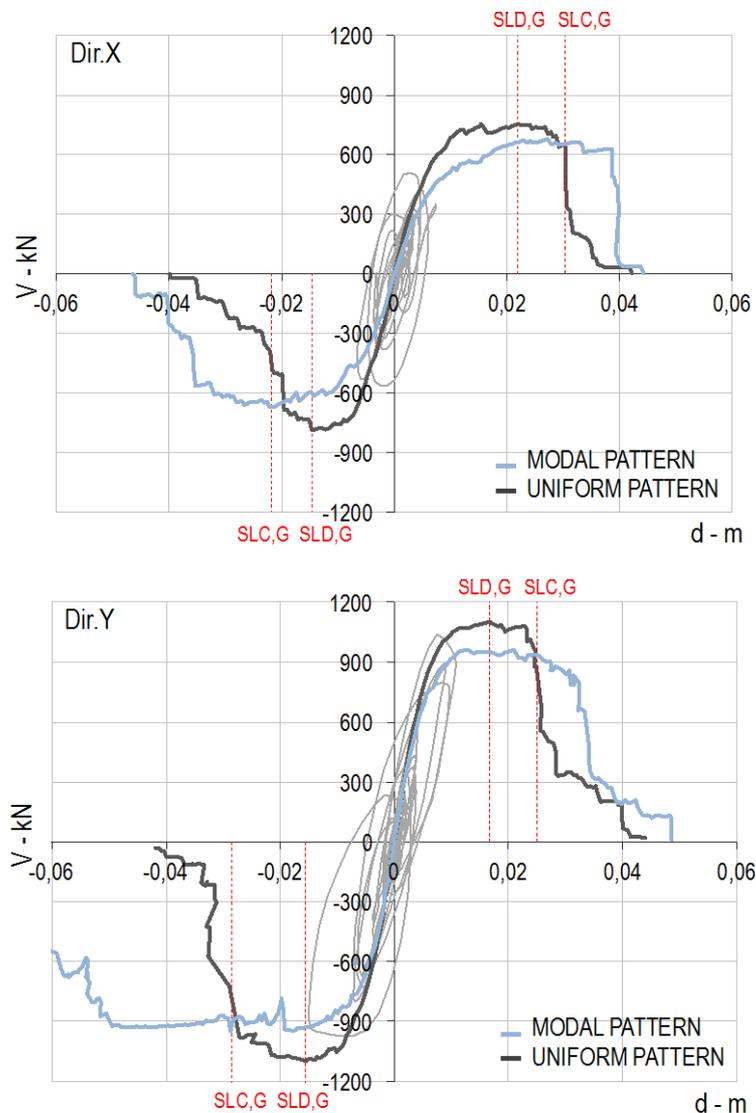
Fig. B-24 Cyclic response in X and Y directions following the application of the event 1, scaled to the value  $S_a(T_1)=6.25 \text{ m/s}^2$  and comparison with the pushover curves obtained from non-linear static analysis.
