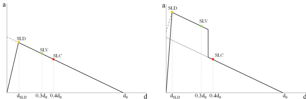
Fig. 3-5. Displacements corresponding to the attainment of various limit states on the capacity curve of local mechanisms: mechanism without resistant elastic-plastic elements (left); mechanism with resistant elastic-plastic elements – tie rods (right).
