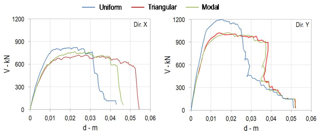
Fig. B-18 Results of the non-linear static analyses in X and Y directions as a function of the various load patterns adopted
