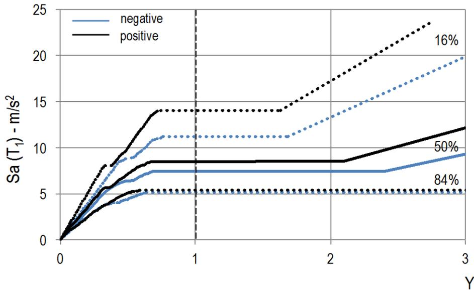
Fig. B-41 ISA curves obtained by comparing the median capacity curve and the median response spectrum (at the 16% and 84% percentiles): Amm-1, X-direction (positive and negative direction) and SLC (which in this case also coincides with SLS).
