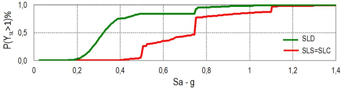
Fig. B-49 Fragility curves for the three limit states, obtained for the first branch of the logic tree (Amm-1).
