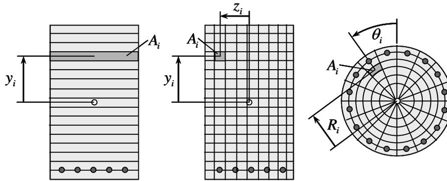
Fig. 4-2 Fiber section models: for plane analyses (left), for spatial analyses (centre and right).
