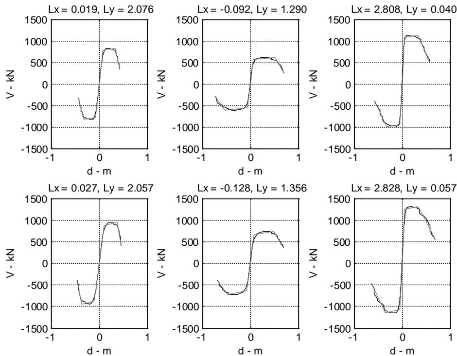
Fig. C -22 Model A: Details of the capacity curves and the corresponding tri-linear approximations for the three significant modes (left to right) and for two of the 30 models sampled (top and bottom).
