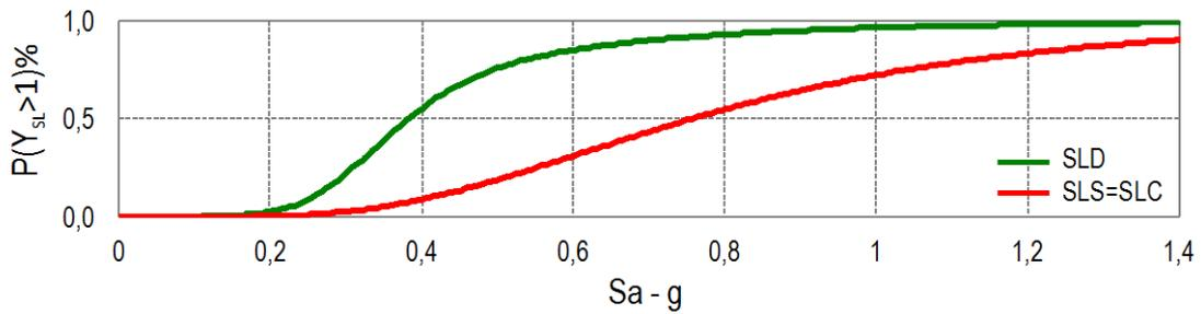
Fig. B-45 Final fragility curves for the three limit states, resulting from the combination of the results obtained in the two branches of the logic tree (Amm-1 and Amm-2).
