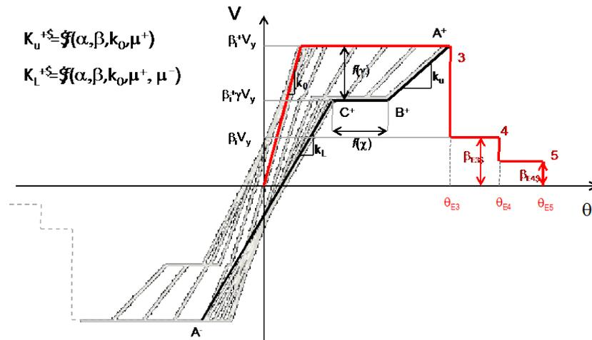
Fig. B -9 Piecewise-linear behavior assumed for masonry panels
