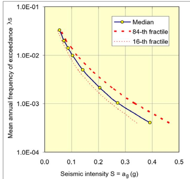
Fig. 2-1 Example of fractile hazard curves (50%, 16% and 84%) for peak ground acceleration  $a_g$ . [Source: Project DPC-INGV S2].
