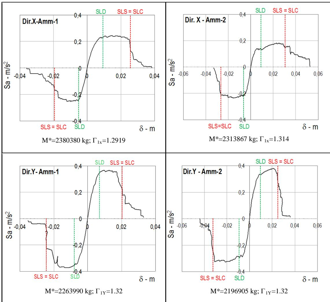
Fig. B-35 Results of non-linear static analyses in terms of capacity curve (conversion of pushover curves into the equivalent single degree of freedom): X direction - positive and negative directions for the two branches of the logic tree (mean values for all the random variables)
