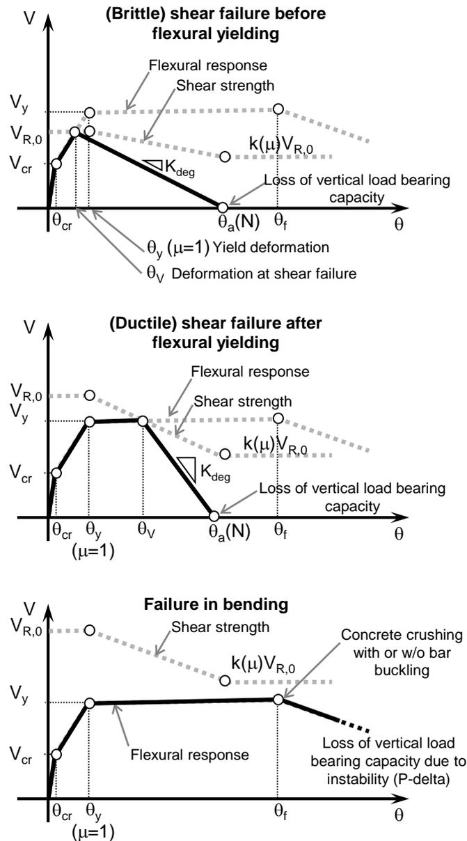
Fig. 4-1 Failure modes of a reinforced concrete element subjected to bending, shear and normal stress
