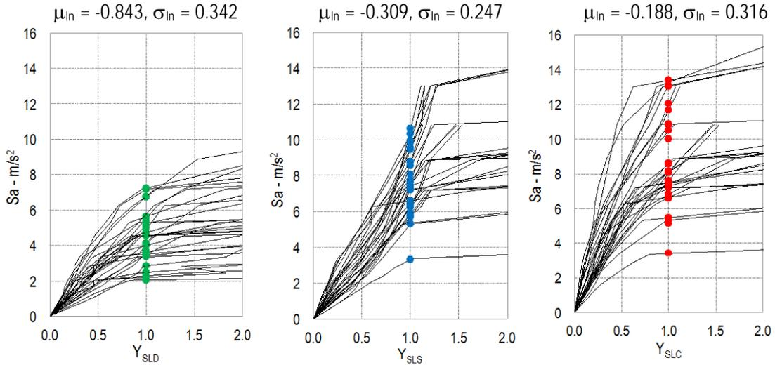
Fig. B-30 Incremental Dynamic Analysis (IDA) curves in terms of limit state variable  $Y_{sl}$  (up above, the parameters that define the lognormal distribution adopted for statistically processing the intensity measures that lead to SLD, SLS and SLC).
