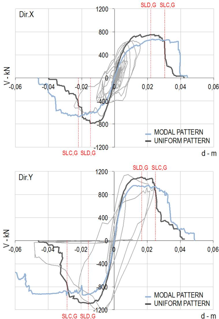
Fig. B-25 Cyclic response in X and Y directions following the application of event 1, scaled to value  $S_a(T_1)=10.84 \text{ m/s}^2$ , and comparison with pushover curves obtained from the non-linear static analysis.
