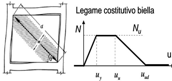
Fig. C -20 Constitutive law of the equivalent rods for infills.
