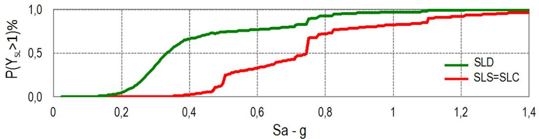
Fig. B-51 Final fragility curves for the three limit states, obtained by combining the results obtained for the two branches of the logic tree (Amm-1 and Amm -2).
