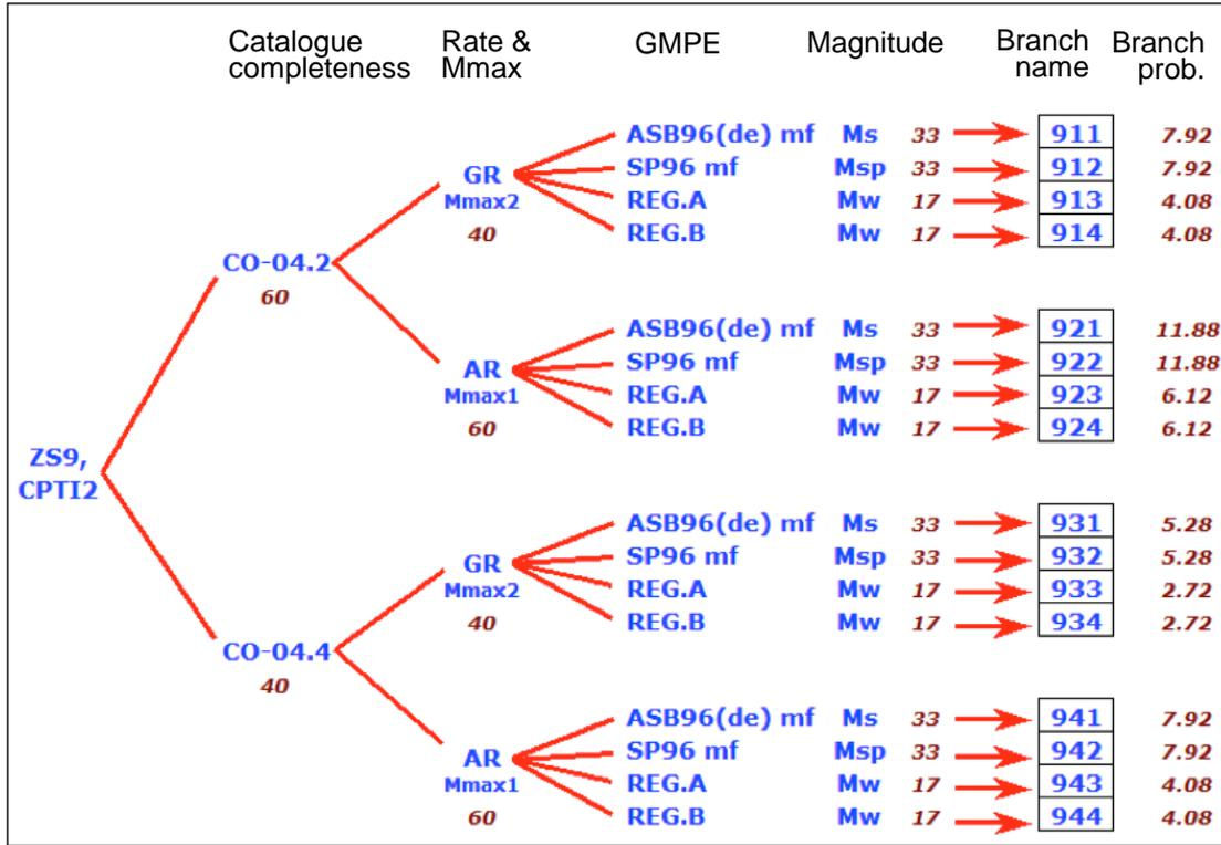
Fig. A-5 Logic tree used in (INGV, 2004) to determine distribution of peak ground acceleration.
