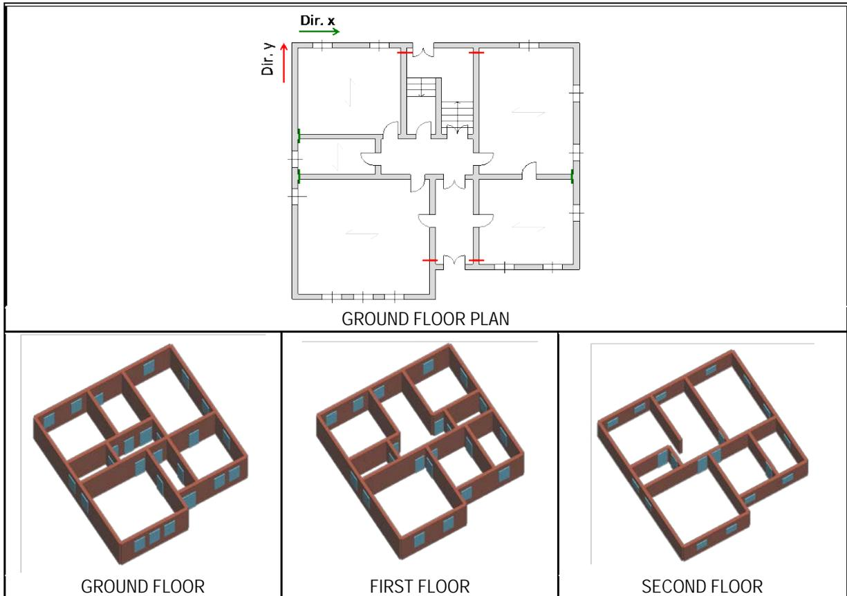
Fig. B-12 Localization on the plan view of the points where the conditions on the wall-to-wall connection were changed and planimetric configuration at the three floors which highlights how some internal walls are not continuous at all levels in X direction (reducing the sensitivity to this factor in particular in the negative sense)
