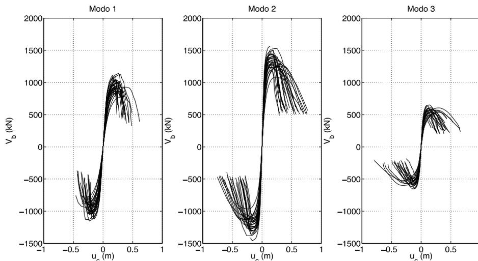
Fig. C-27 Model C: Dispersion in capacity curves for the three significant modes.
