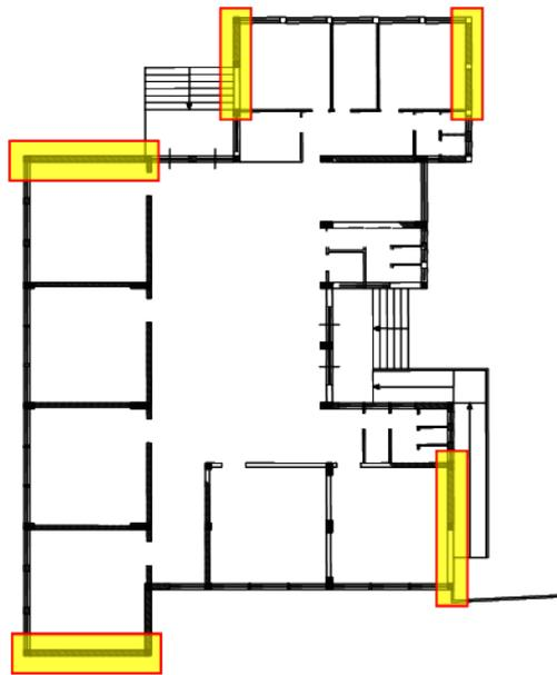
Fig. C-12 Distribution of the infills in plan.
