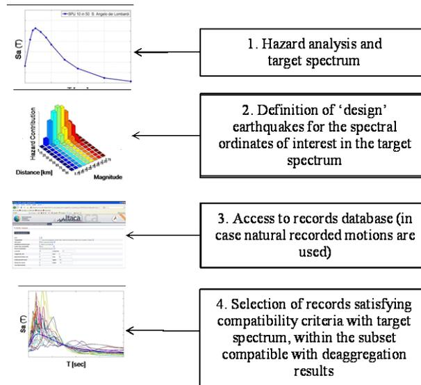
Fig. A-6 Fundamental steps in the process of selection of seismic motion time histories.
