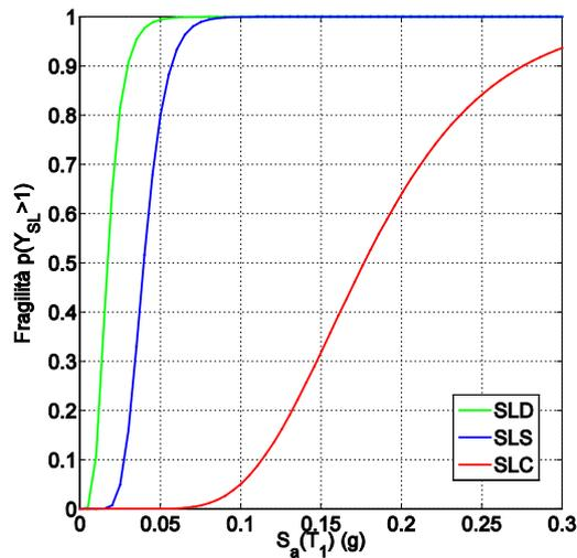
Fig. C-30 Model B: Fragility curves for the three SL.
