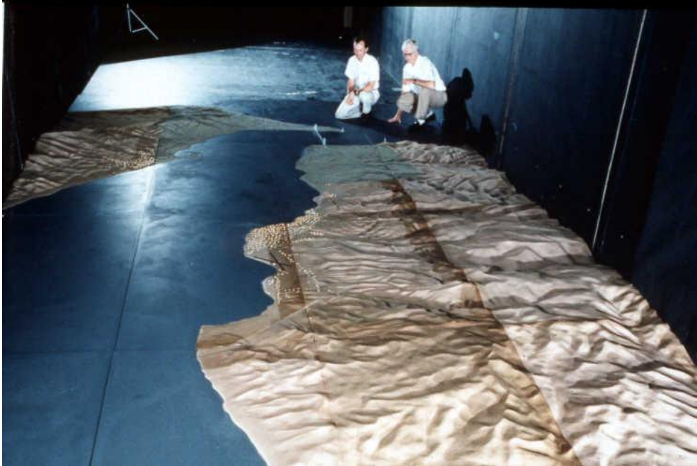
Figure Q.2 – Wind field modelling test over complex orography.
