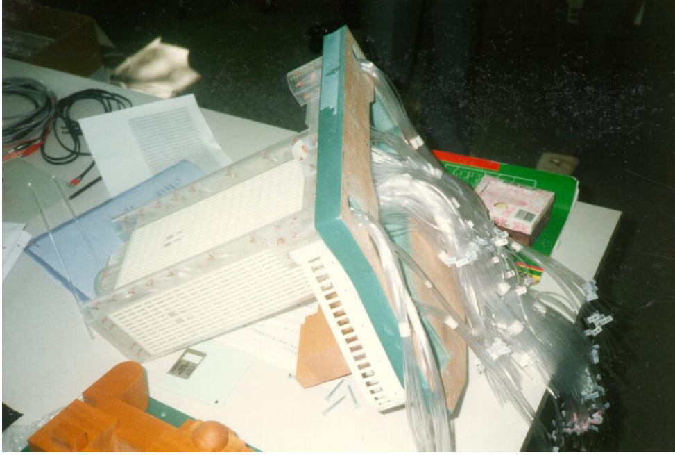
Figure Q.3 – Pressure model with tubing.
