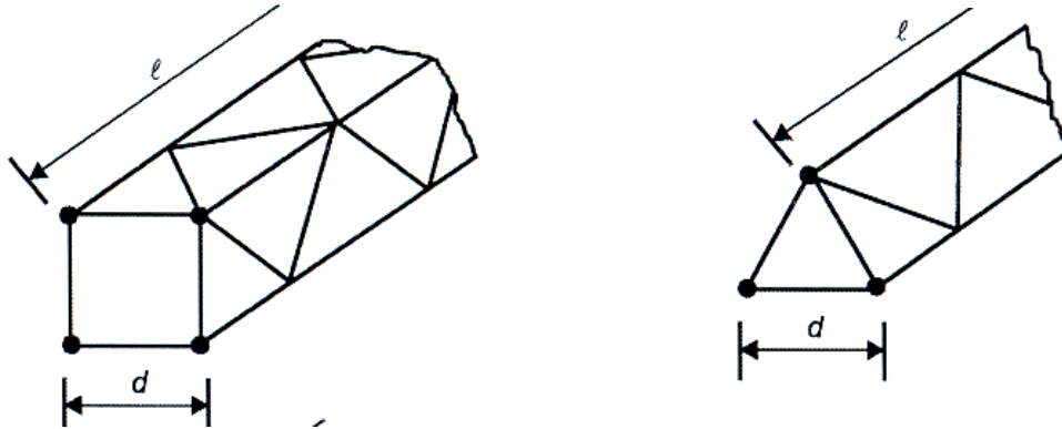
Figure G.43 – Characteristic dimensions of lattice girders.
