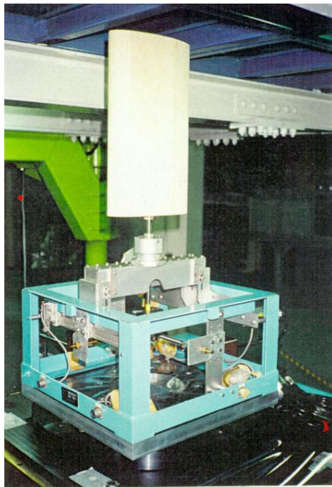
Figure Q.9 –Building pivot model test.
