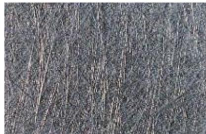
Discontinuous fibers *mat*.**Figure 7-5** – Fiberglass *mat*.
