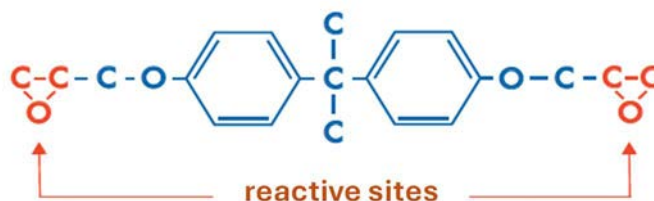
Figure 7-17 – Chemical structure of an epoxy oligomer based on diglycidyl ether of bisphenol A (DGEBA).
