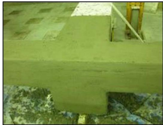
Figure 2.16 – Strengthening of beam-columns joints with unidirectional galvanized steel fibre strips and mortar.
