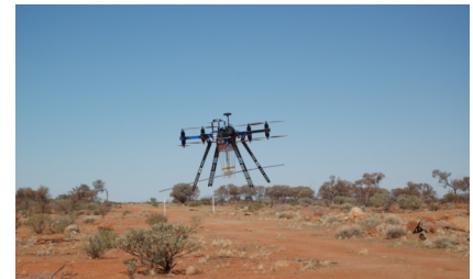
UAV equipped with a VHF synthesizer and dipole antenna operated as a test source for station prototypes of the Square Kilometer Array.
