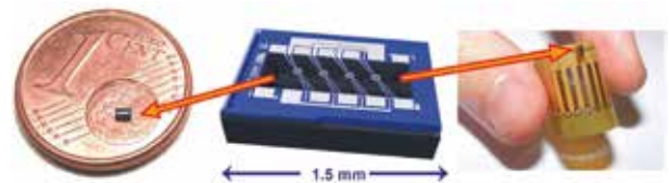
- Ultra-low-power MOX gas sensor array: size compared to a 1 eurocent coin (left), and sensor array flip-chipped on a flexible PCB (right)
