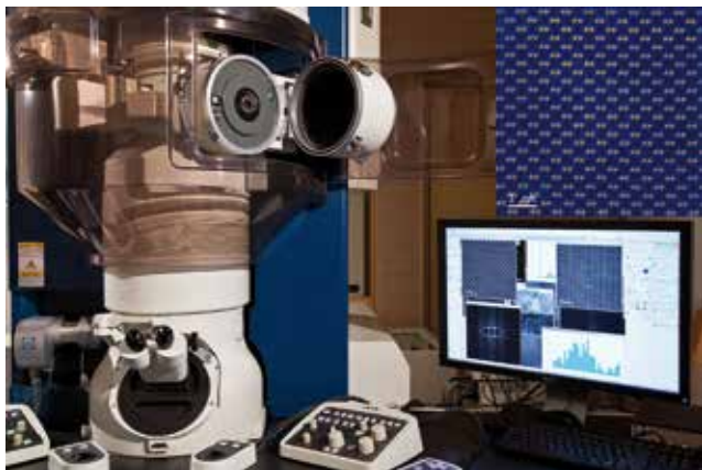
- JEOL ARM200F at the Beyond Nano Microscopy Lab. On the right, structural image of a Si substrate.
