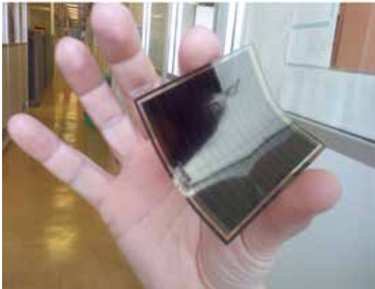
- Amorphous-Si PV mini-module on flexible substrate (polyimide) realized in collaboration with STMicroelectronics.
