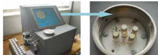
- Electronic nose prototype (left) and zoom on the Sensor Array.
